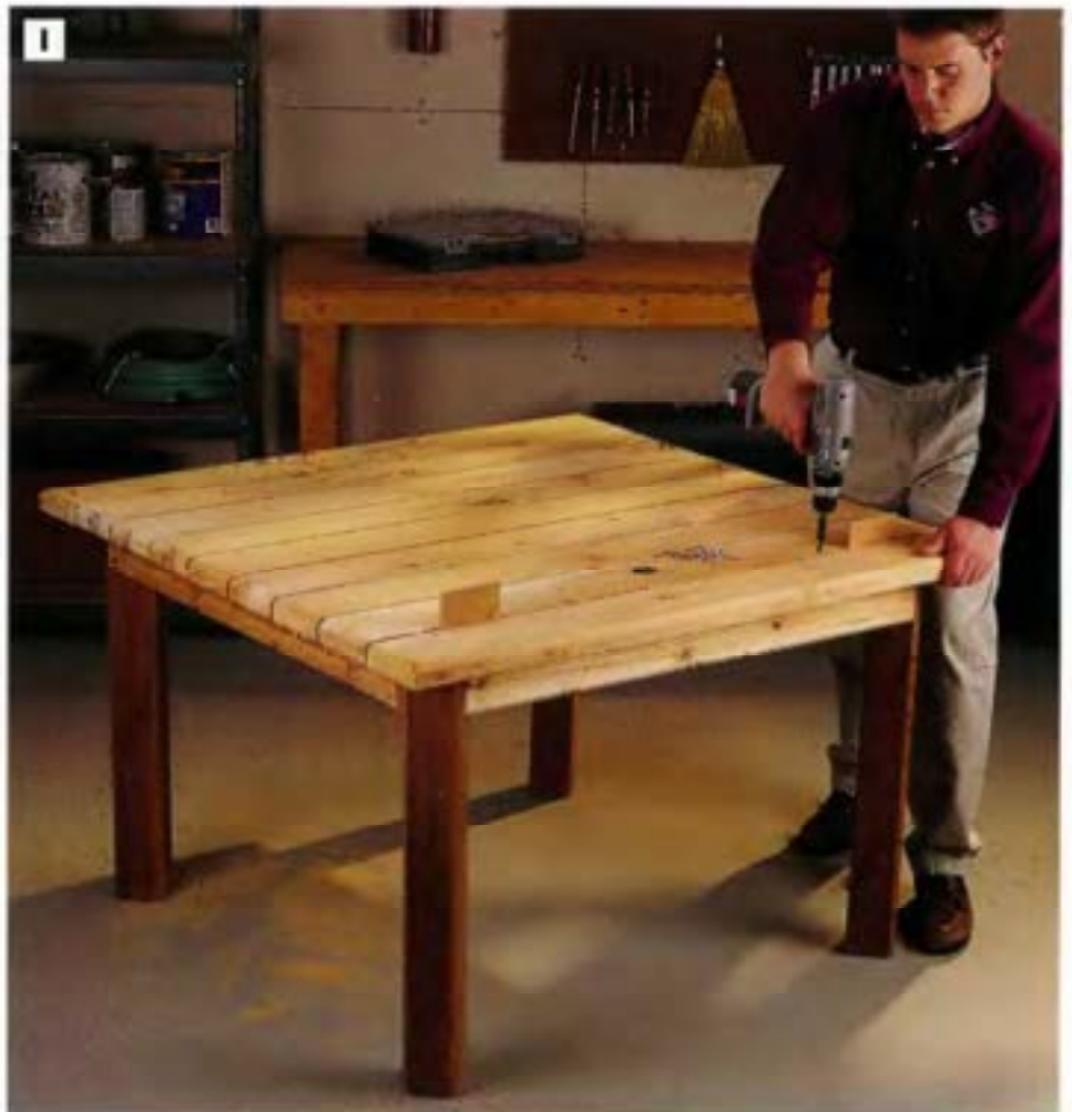
PHOTO I: Attach the top slats to the aprons with 2½-in. deck screws. Fasten the center slat first, then work outward. This way, the overhang will be consistent on both ends of the table, and the slats will be evenly positioned. Use a pair of \frac{3}{16} -in. spacers to create uniform gaps between the slats.
