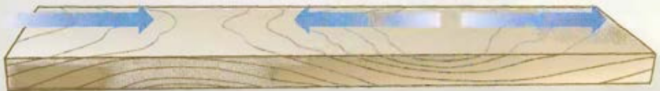
Wavy grain: Switch directions to plane toward crests
