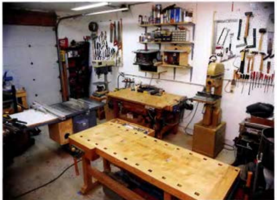
THE GARAGE SHOP: The garage, especially one attached to the house, offers the convenience of a basement shop with fewer drawbacks. Overhead doors provide excellent access, greater headroom, lower humidity and better ventilation. The main general drawback is that garages are usually home to one or more vehicles and a host of other outdoor items. A good solution is to mount your stationary tools on casters so they can be wheeled out of the way to make room for other things.
