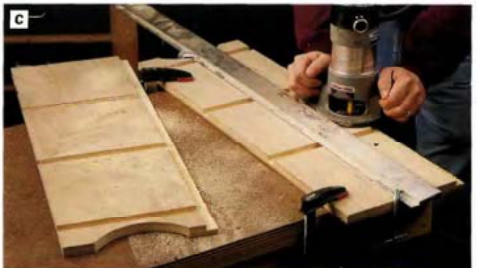
PHOTO C: Rout \frac{3}{4} -in.-wide, \frac{3}{8} -in.-deep rabbets along the inside back edge of each side panel for the bookcase back. Clamp each side panel to your bench to hold it securely as you rout the rabbet, and guide the router base against a straightedge.
