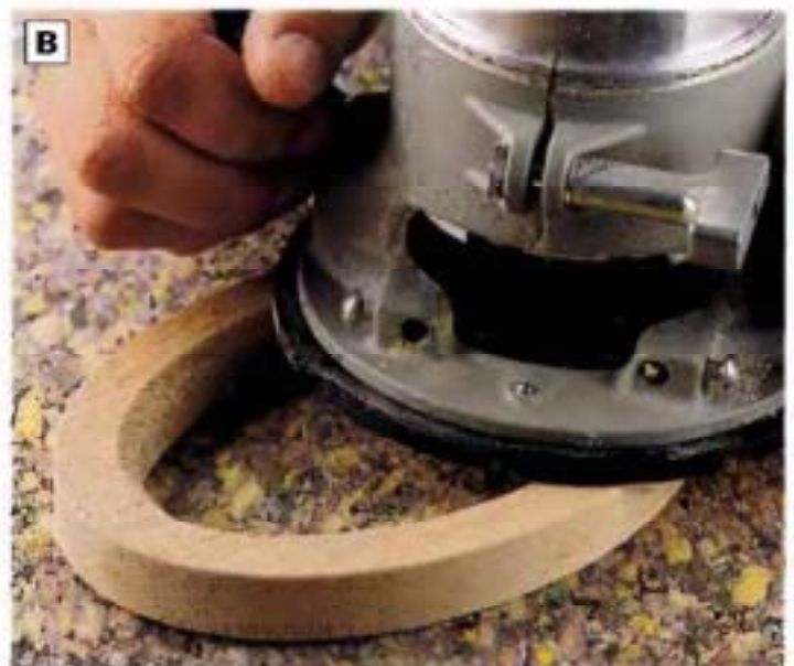
PHOTO B: Mill the 45° chamfer on the inside edge of the frame with the router held free-hand. Use a non-slip pad beneath the workpiece while you rout. Then turn the frame over, switch to a \frac{1}{4} -in. piloted rabbeting bit and rout the back rabbet around the inside edge.
