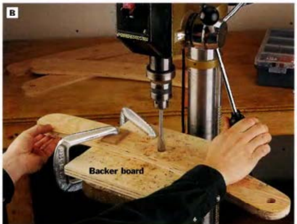
PHOTO B: Bore the \frac{3}{4} -in.-dia. leg pivot and lock dowel holes in the legs. These holes must be drilled straight through the legs, or the dowels will be difficult to align during assembly. Bore the holes with a drill press, or mount your drill/driver in a right-angle drill guide. Set a backer board beneath each workpiece before you drill, to keep the bit from tearing out the wood as it exits.
