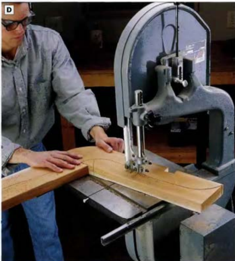
PHOTO D: Use a template to transfer the patterns of the back supports and seat supports onto the glued-up blanks, and cut out the shapes with a band saw or jig saw.
