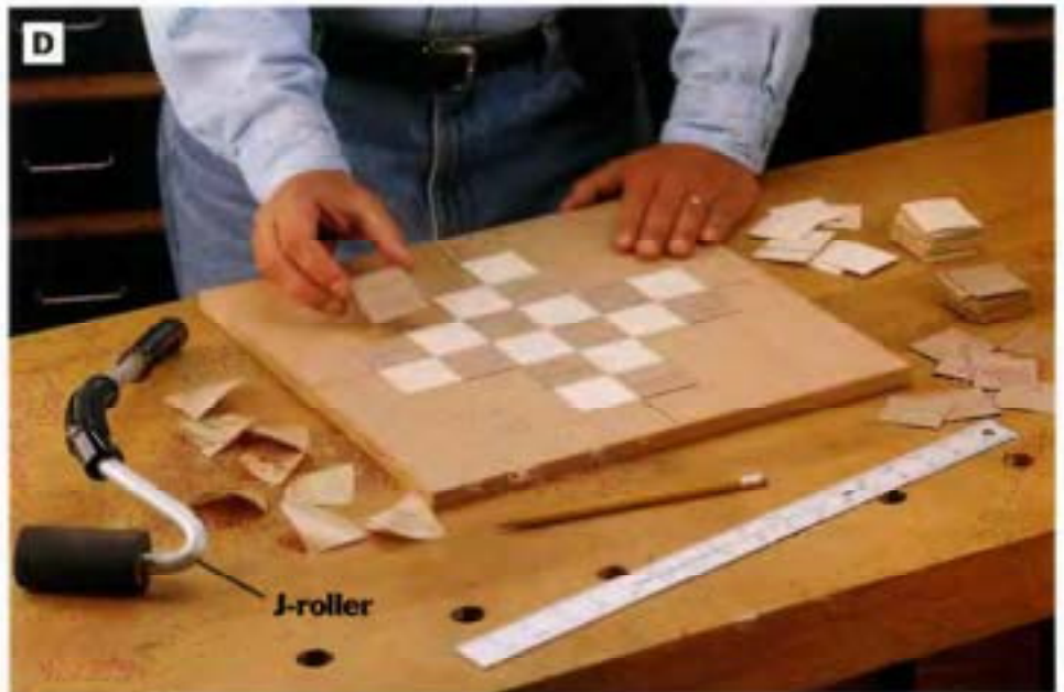
PHOTO D: Divide the MDF top panel into four layout quadrants with a straightedge and pencil. Then begin to install the veneer squares, starting with a group of four at the center. Work outward from the center, in all four directions, fitting the squares as tightly together as you can. Use a J-roller or rolling pin to press the back of each square firmly in place.
