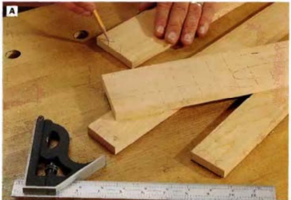
PHOTO A: Lay out the finger joints on the ends of the tray side and end pieces. Use a combination square to mark the joints. Draw X's on the waste areas.
