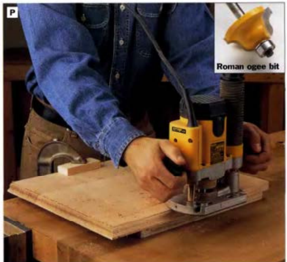
PHOTO P: Clamp the top panel to the workbench and use a Roman ogee bit to rout a profile around the side and front edges. Insert scrap plywood between the benchtop and the top panel to give clearance for the bit's pilot bearing.
