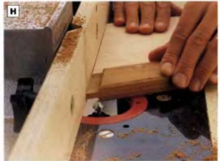
PHOTO H: Rout ⅜-in. chamfers on the ends and edges of the slats using a V-groove bit in the router table. Use an angled pushblock to guide the workpiece.
