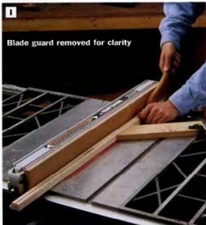
PHOTO I: Rip the cove molding for the cupboard crown to width on the table saw. Use a featherboard and pushstick.
