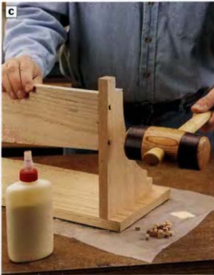
PHOTO C: Once you've attached the coatrack parts, cover the screw heads with face-grain red oak plugs held in place with glue. Tap each plug into its counterbore with a wooden mallet.
