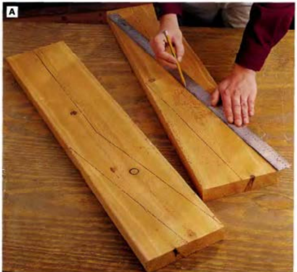
PHOTO A: Lay out and cut eight back chair legs to shape. Use the Back Legs drawing, page 389, to establish reference points for drawing the leg shapes. Connect the points with a straightedge.
