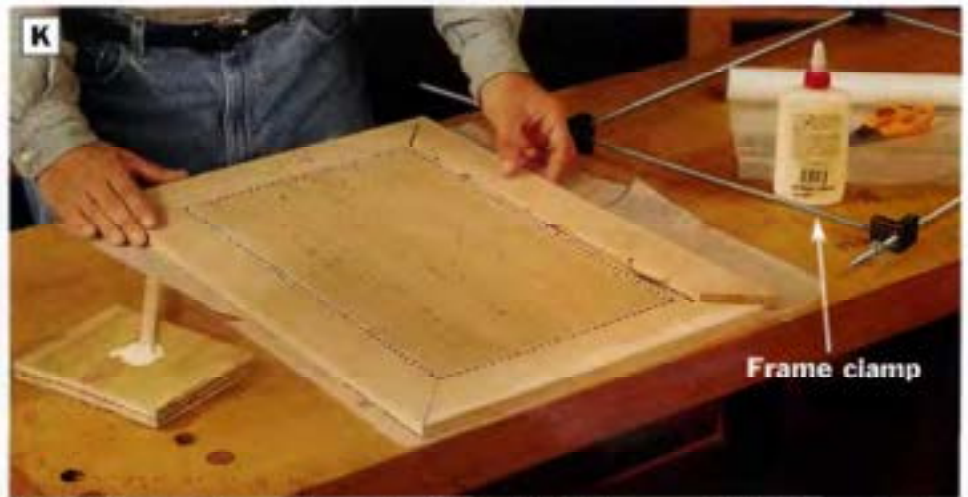
PHOTO K: Attach the frame sides and ends to the inlaid bottom panel with glue and biscuits. Dry-fit the parts together first with the biscuits in place. Once the pieces are glued and fitted, install a frame clamp around the assembly and tighten.
