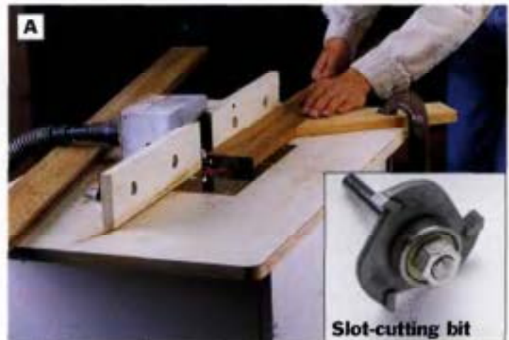
PHOTO A: With a slot-cutting bit (See inset photo) in the router table, rout a \frac{1}{4} -in.-wide \times \frac{1}{2} -in.-deep groove into the edge of the tabletop rail stock. Use a featherboard to hold the stock against the fence.
