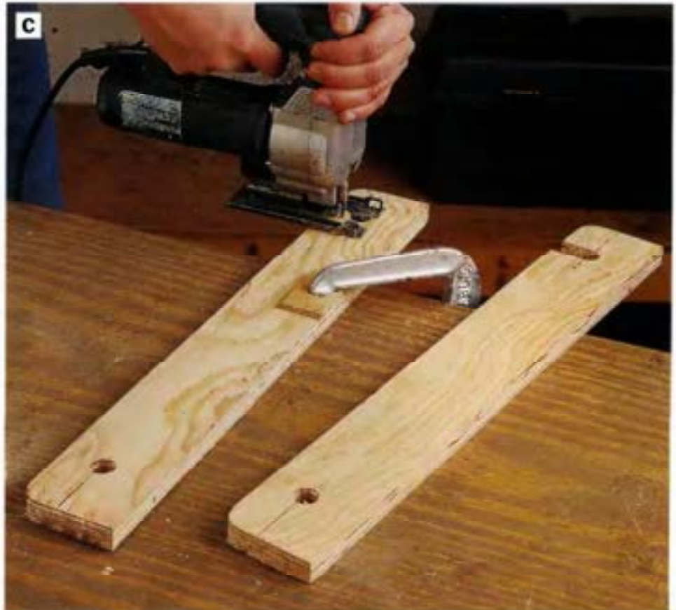
PHOTO C: Connect the lock dowel hole with straight lines to the edge of each stretcher, forming the lock dowel slots. Clamp the legs to your worksurface and cut along these lines. The width of the slots should be \frac{13}{16} in., to provide a loose fit for the \frac{3}{4} -in.-dia. lock dowel.
