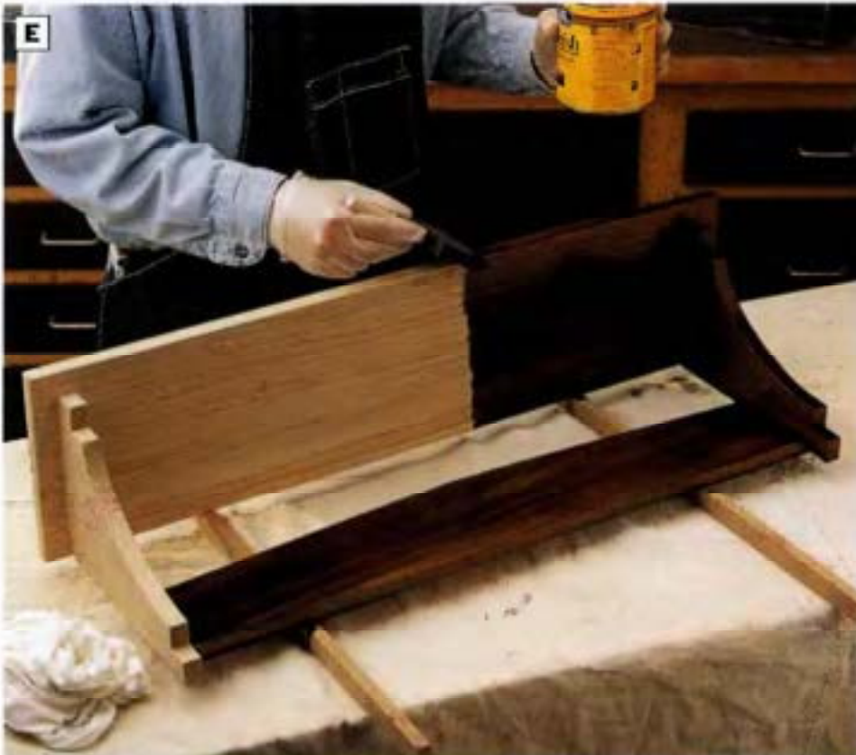
PHOTO E: Brush or wipe on a coat of wood stain with a foam brush or clean rag, then wipe off the excess stain before it dries. Wear disposable gloves to protect your hands. Topcoat the project with varnish.
