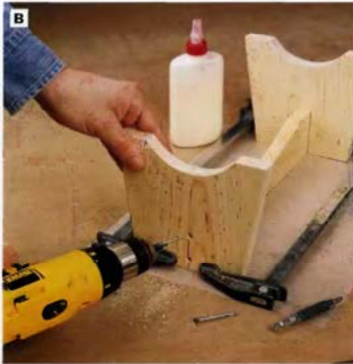
PHOTO B: Glue and clamp the stretcher between the legs so the top ends and edges of the parts are flush. Fasten the parts with countersunk 2-in. flathead wood screws.
