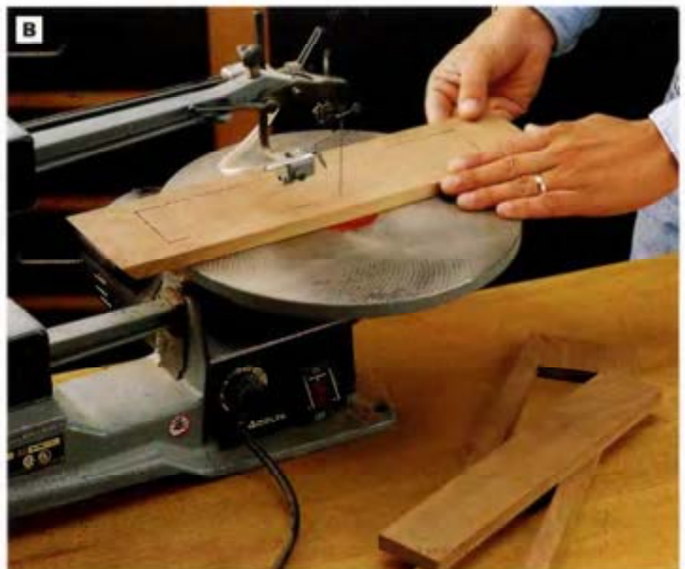
PHOTO B: After drilling starter holes at all four corners of both drawer faces, carefully cut out the faces from the front and back workpieces. The faces are cut from the front and back parts so the wood grain will match when the drawers are closed.
