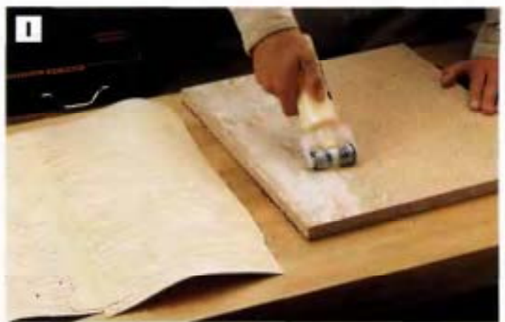
PHOTO I: Apply an even, light coat of glue to the unfinished particleboard face of the melamine board. Because the glue sets up quickly, have the veneer and your veneer press close at hand.
