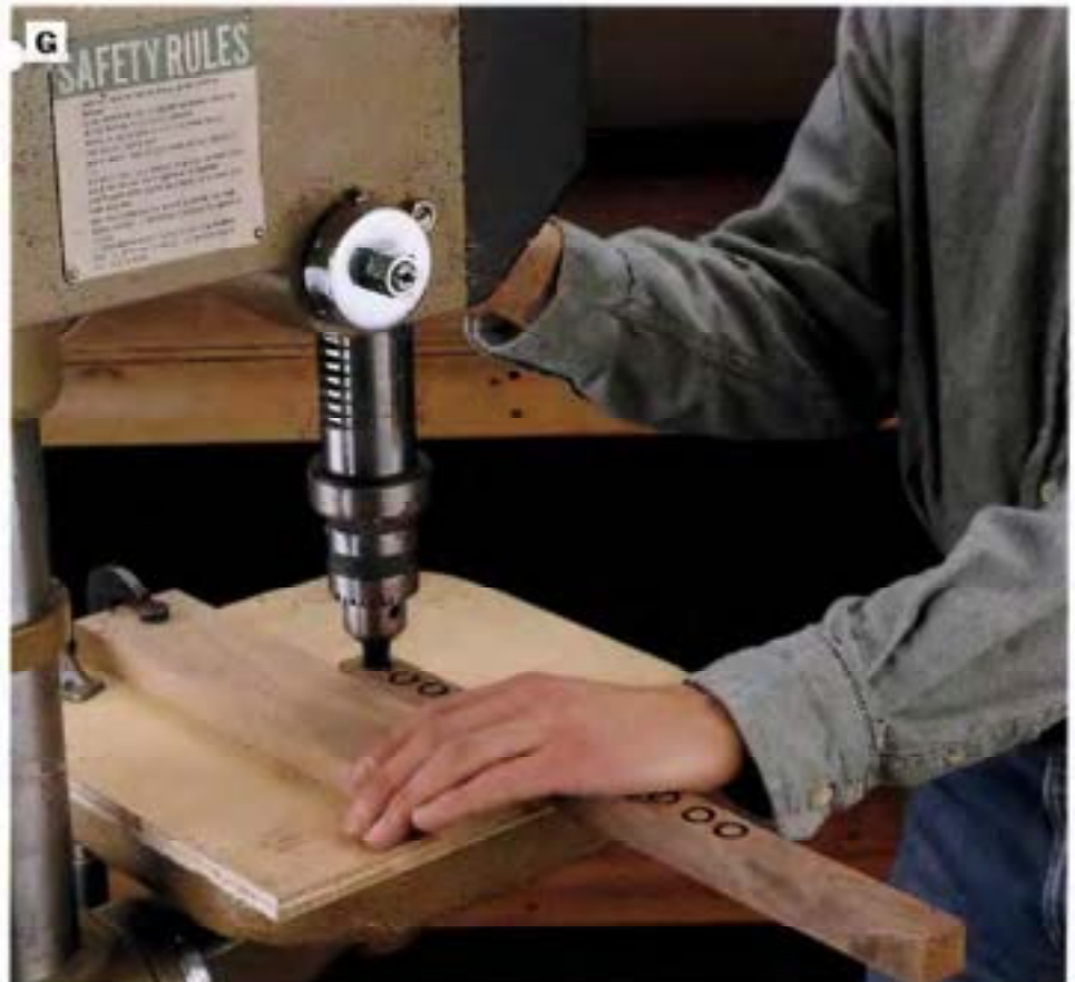
PHOTO G: Make walnut screw plugs on the drill press, using a \frac{3}{8} -in. tapered plug cutter. Clamp a scrap piece to the drill press table to create a surface that helps keep the walnut stock stationary while you cut the plugs.
