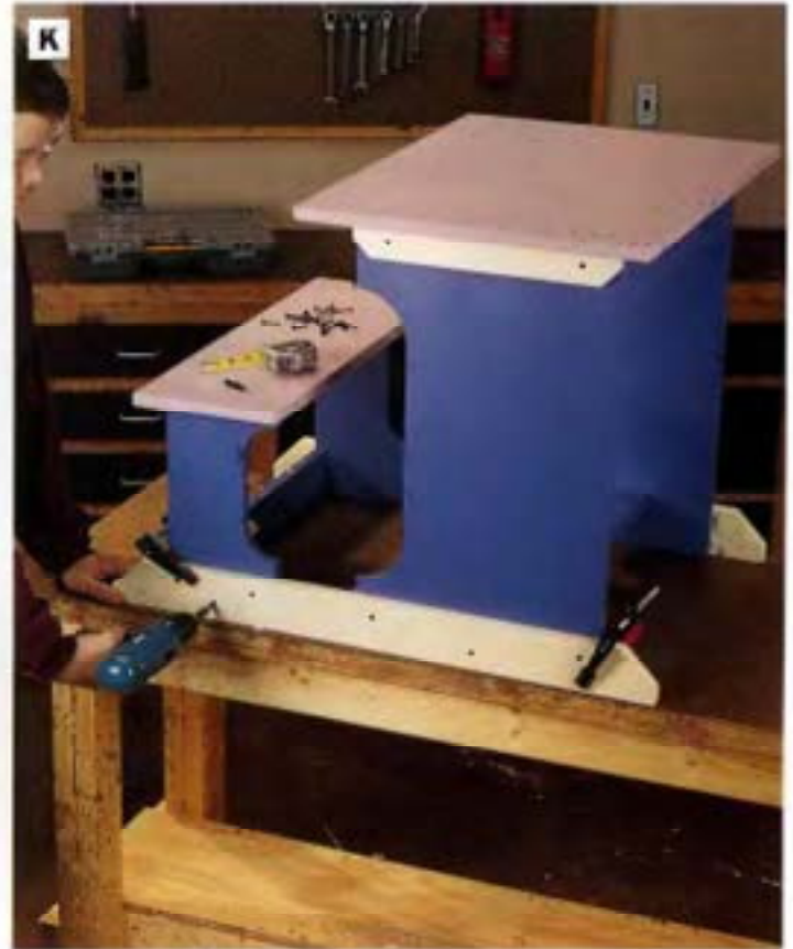
PHOTO K: Fasten the runners to the bench and desk legs with countersunk 1¼-in. drywall screws. Hold the parts together with clamps while you drive the screws. Stagger the screw pattern.
