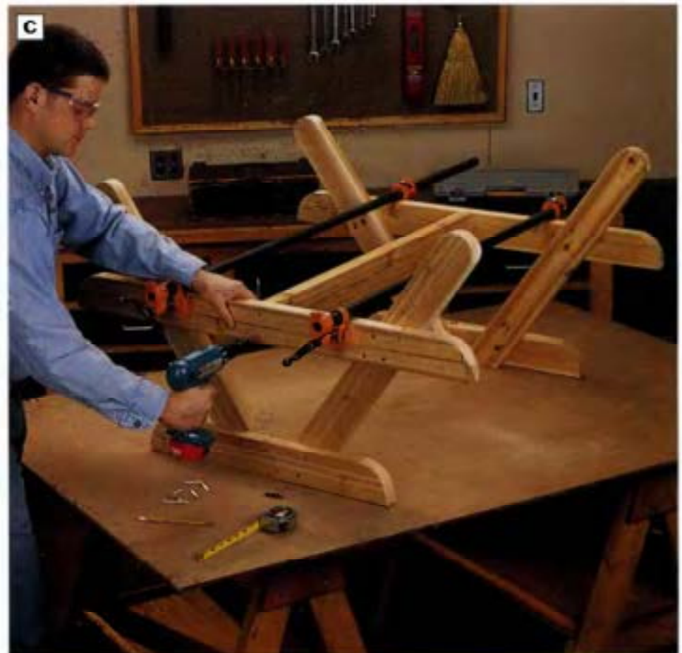
PHOTO C: Stand the leg assemblies top-down to attach the stretcher between them. Hold the stretcher in place with clamps so it is centered on the length of the seat stringers. Drive countersunk 3-in. screws through the seat stringers and into the ends of the stretcher.
