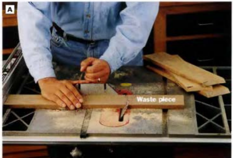
PHOTO A: Crosscut the front, back and side pieces to length on the table saw with the blade tilted to 45^\circ . Since all four parts are the same length, you can use the saw fence as an index to establish the length of the parts, like we show here. CAUTION: If you use this method, the blade must tilt away from the fence, and the waste piece must fall away on the side of the blade opposite the fence. Otherwise, the waste piece or the workpiece could become trapped between the blade and the fence and result in kickback.
