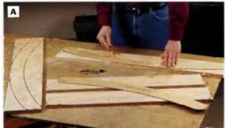
PHOTO A: Create seat and back support templates from hardboard, and use these templates to draw the profiles on the back and seat support workpieces (use treated lumber, not plywood as shown). Cut out the parts with a jig saw.
