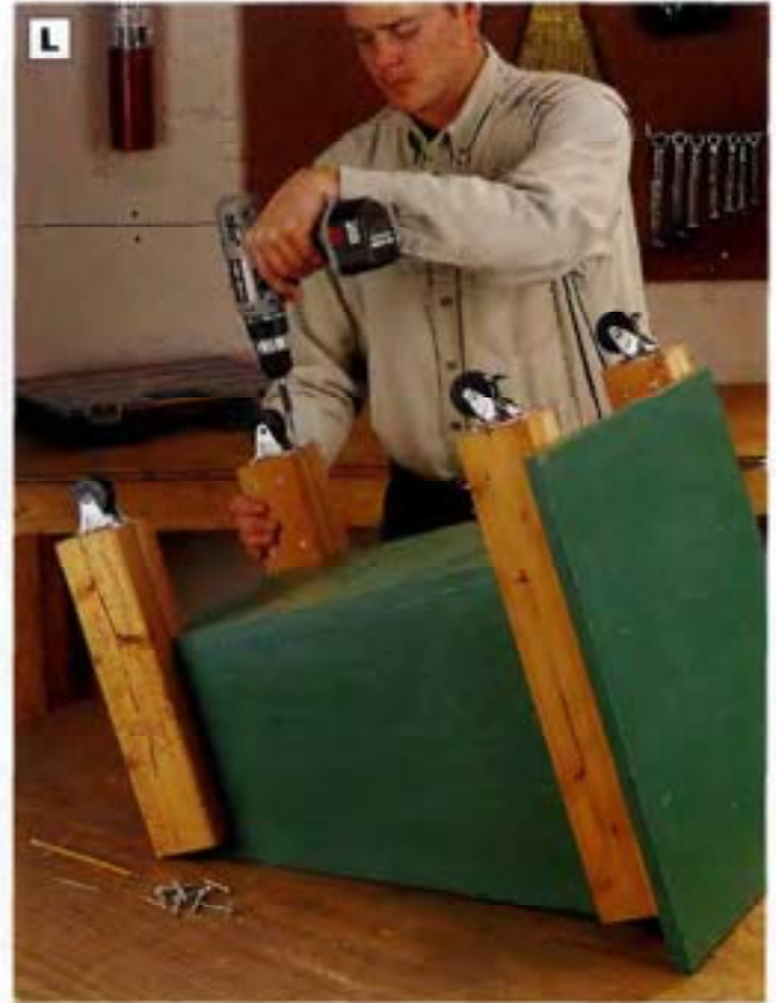
PHOTO L: Attach casters to the cart leg and cleat assemblies. We used swiveling locking casters on the front legs and fixed casters on the back. If you plan to fill the cart with dirt, be sure the casters are sturdy.
