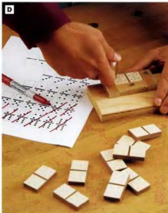
PHOTO D: Mark the dot locations on the domino blanks, using the Tile Holes & Centerlines pattern drawing on page 289 as a guide. For greater precision, we built a simple jig with a clear Plexiglas top drilled with \frac{1}{16} -in.-dia. holes at each dot location. We pressed a finish nail through the appropriate holes in the Plexiglas to mark each dot pattern.
