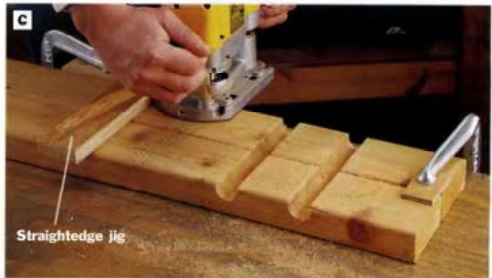
PHOTO C: Gang-rout notches in the back supports to ensure that the notches will line up perfectly on both pieces. Use a ¾-in. core box bit, and cut the notches in several passes of increasing depth. We clamped a short T-square style straightedge jig to guide the router when cutting.
