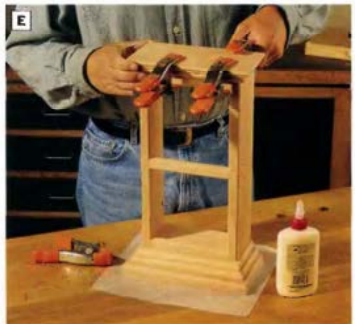
PHOTO E: Glue up the crown and base first, then glue these completed assemblies to the clock carcass. Glue alone will bond these parts sufficiently, so no additional fasteners are needed.
