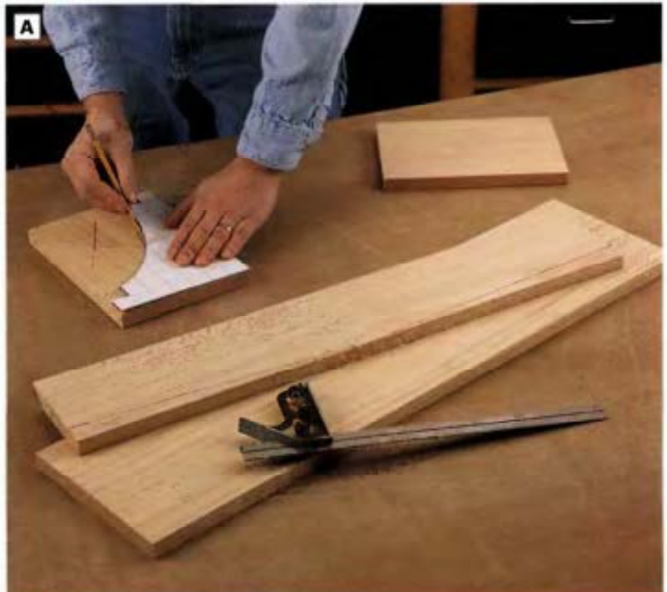
PHOTO A: Lay out the tapered profile on the back panel with a straightedge, and use a full-size paper or cardboard template as a guide for drawing the curved end profiles.
