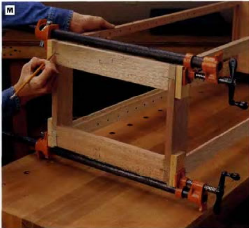
PHOTO M: Clamp up the cabinet frame temporarily and mark the biscuit locations on the top supports and side panels. Disassemble the cabinet and cut slots for #20 biscuits.
