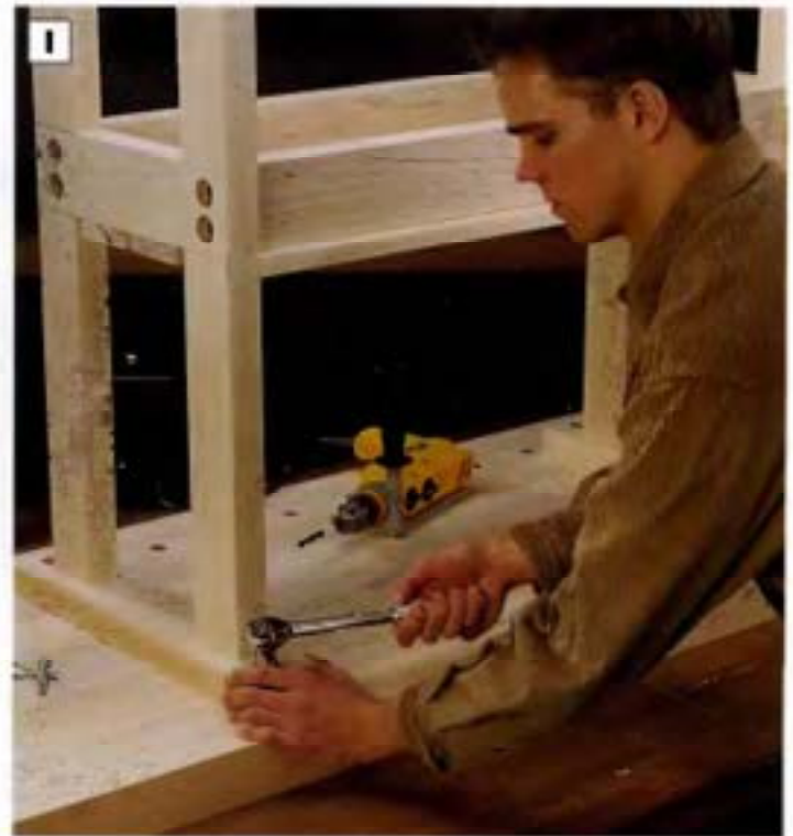
PHOTO I: Center the base on the underside of the benchtop, then attach it with lag screws driven through the top supports.
