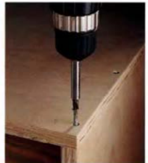
WOOD SCREWS are popular fasteners for reinforcing butt joints. They should be driven into counterbored or countersunk pilot holes.
