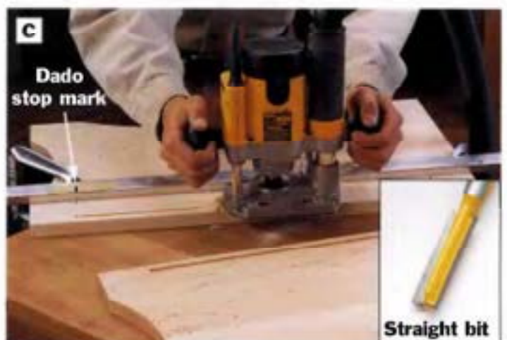
PHOTO C: Rout \frac{1}{4} \times \frac{1}{4} in. dados along the inside faces of the sides, \frac{1}{2} in. in from the back edges, using a \frac{1}{4} -in. straight bit (See inset photo). Stop the cuts 2\frac{1}{2} in. from the bottom edges of the sides.
