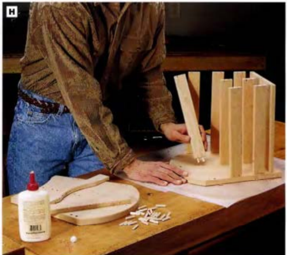
PHOTO H: Glue the dowels in the ends of the handle, the slats, and the bottom into the corresponding dowel holes in one side panel. Then immediately glue dowels into the other end panel and set it onto the upright ends of the parts. Align the dowels into their holes and press the assembly together.
