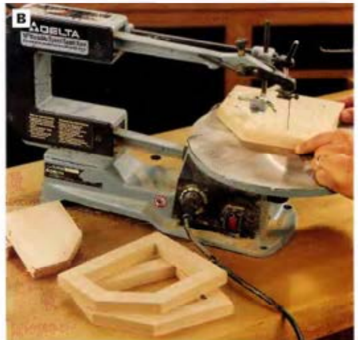
PHOTO B: Lay out and cut one frame to shape on the scroll saw, then use this first frame piece as a pattern for tracing the shapes of the other seven frames. To remove the center cutout from each frame, drill relief holes at each corner of the cutout so you can turn the workpiece on the scroll saw as you cut.
