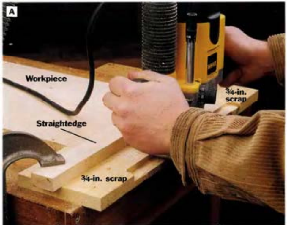
PHOTO A: Cut \frac{3}{4} \times \frac{3}{8} -in.-deep rabbets in the top and bottom of the side panels for the upper cabinet, and cut \frac{3}{8} \times \frac{3}{8} -in.-deep rabbets in the top and bottom of the side panels for the lower cabinet. Also cut \frac{3}{8} \times \frac{3}{8} -in.-deep rabbets in the ends of the top and bottom panels for the lower cabinet. Use a router and straight bit to make the cuts. Clamp pieces of \frac{3}{4} -in.-thick scrap on each side of the workpiece, and clamp a straightedge cutting guide for the router to follow.
