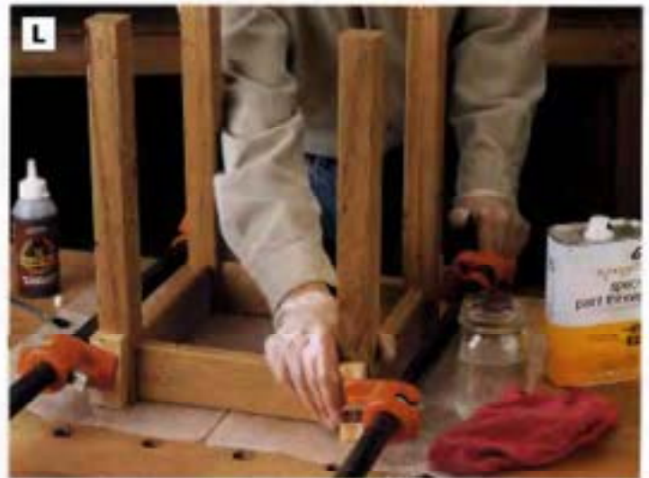
PHOTO L: Glue and clamp the legs and rails together. Use clamp pads between the clamp jaws and mineral spirits to clean up squeeze-out.
