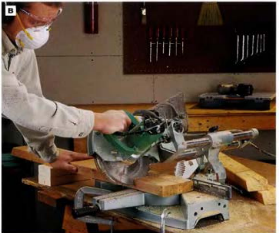
PHOTO B: Bevel-cut the ends of the outer and center table stretchers at 30° angles. We used a power miter box, but you could also make these cuts with a circular saw or a table saw.
