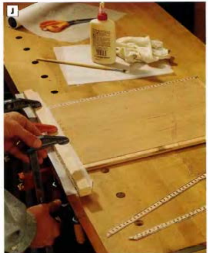
PHOTO J: Install the inlay strips on the bottom panel rabbets. Glue one piece at a time to the plywood, and press it firmly in place with a couple of clamps and a wood caul. Cover the inlay with wax paper before clamping on the caul to keep the parts from sticking together.
