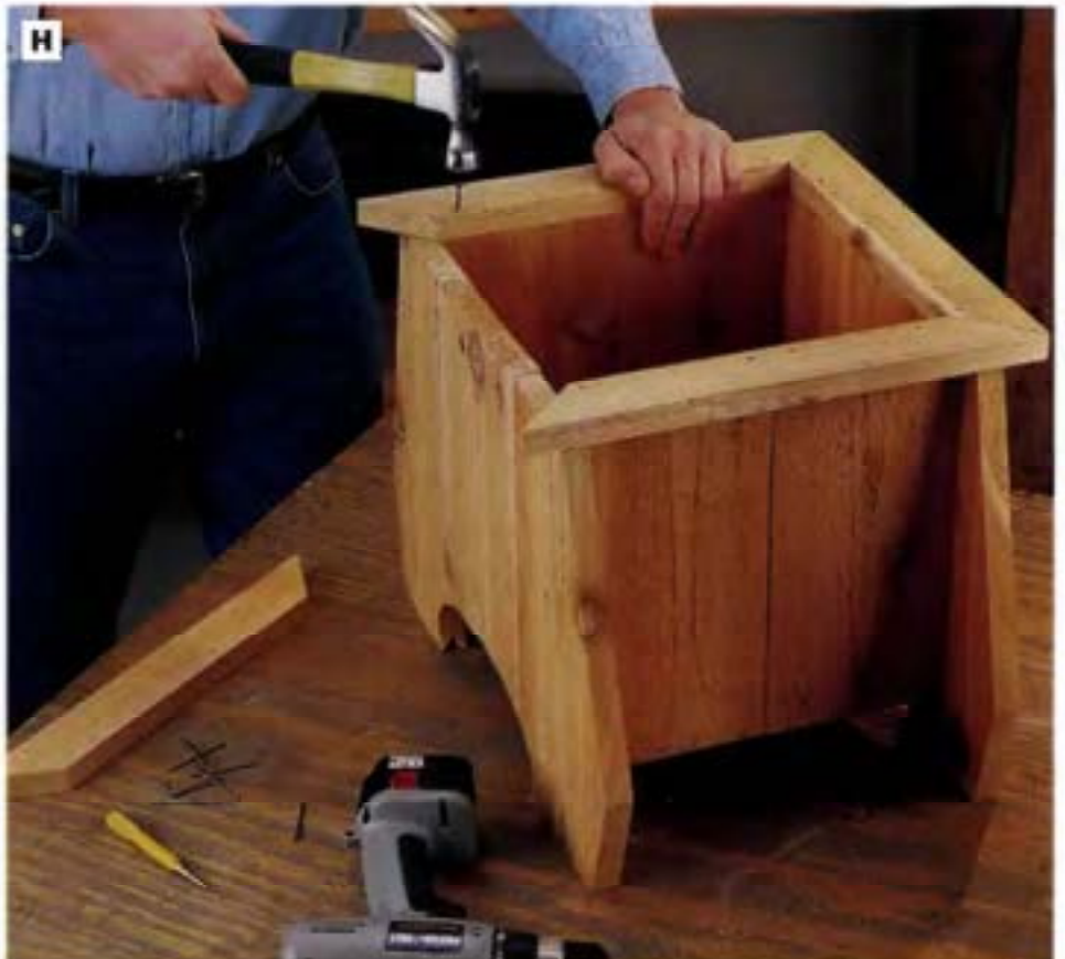
PHOTO H: Install the four crown pieces around the top of the planter with nails. Lay out and cut the crown pieces so they are mitered on the ends and fit flush with the inside of the planter.
