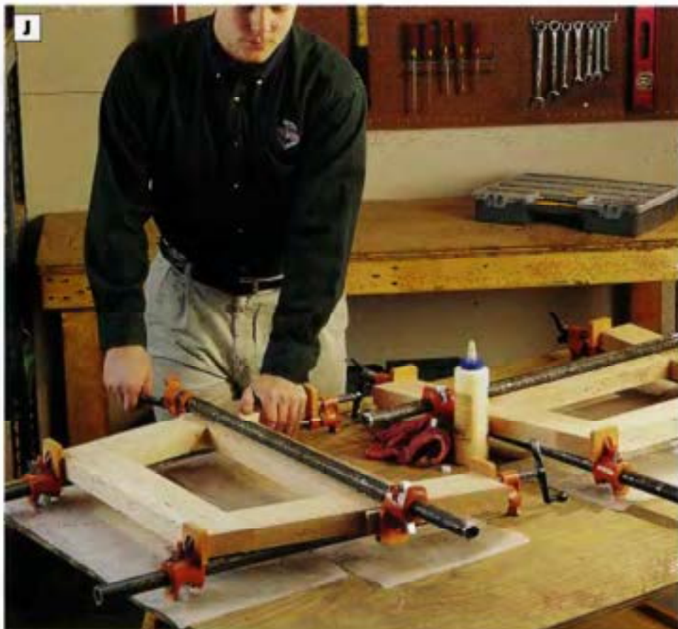
PHOTO J: Build the glider stand ends by attaching the top and bottom end rails to the stand legs with dowels and glue. The bottom rails fit between the legs, while the top rails overlap the top ends of the legs.
