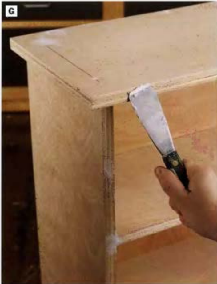
PHOTO G: Conceal the screwheads and any voids or gaps in the plywood with wood putty. Sand the putty smooth when it dries.
