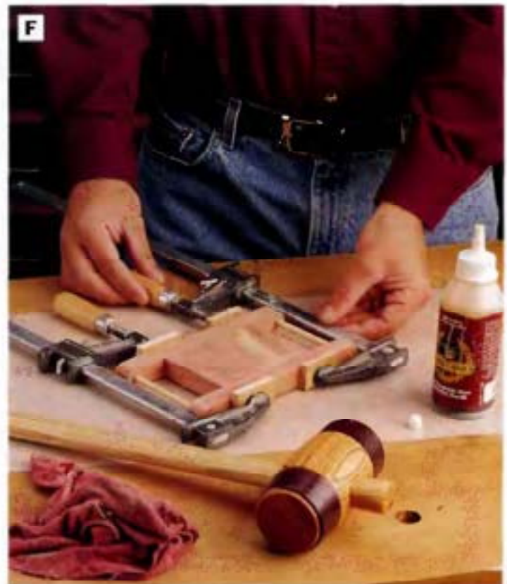
PHOTO F: Assemble the base plate, base strips and perches with polyurethane glue. Clamp the parts together to keep the glue from forcing the joints open as it cures.
