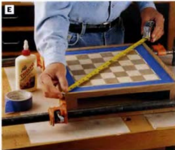
PHOTO E: Assemble the top and bottom, front, back and sides with #0 biscuits and glue to form the carcass. Protect the perimeter of the veneer top from glue squeeze-out with masking tape. Be sure the carcass is square when you clamp by measuring the diagonals. When the diagonal measurements match, the carcass is square. Adjust the clamps, if needed, to adjust for square.
