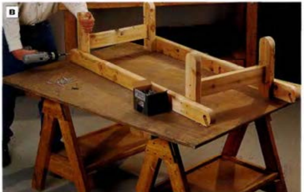
PHOTO B: Fasten the leg assemblies to the seat rails with 2\frac{1}{2} -in. galvanized deck screws. Be sure the foot rest notches on the seat rails face down on your worksurface when you fasten the legs to the rails. Check the leg assemblies with a square to be sure they are perpendicular to the rails before driving the screws.
