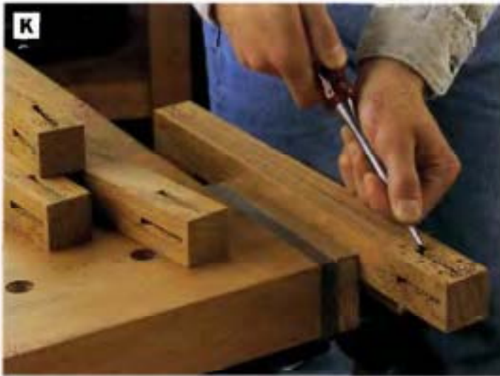
PHOTO K: Drill out the leg mortises on the drill press to 1/2-in. depth. Clean up the waste from the shoulder of the mortises with a chisel.
