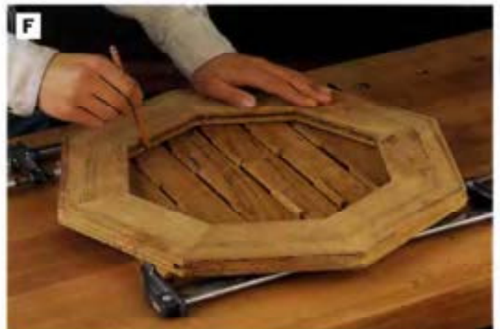
PHOTO F: Insert \frac{1}{4} -in. spacers between the slats and clamp them together. Lay the rail assembly over the slats and trace the interior of the assembly onto the slats.
