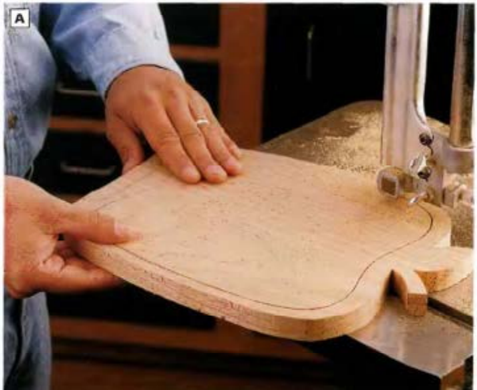
PHOTO A: Cut out the apple-shaped frame that supports the basket. Then mark and cut out the basket from the center of the frame as well as the stand.
