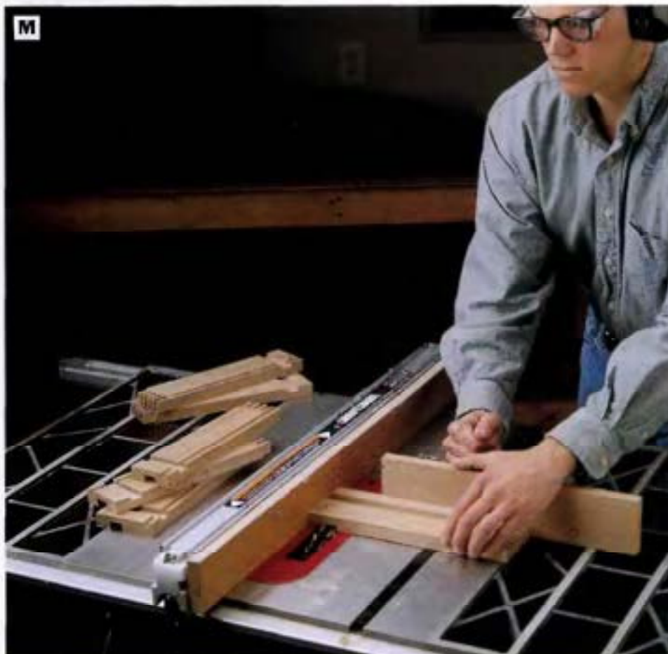
PHOTO M: Cut the drawer back dados on the table saw with a dado blade, miter gauge, and rip fence. Push the stock across the blades carefully to avoid binding the workpiece between the blades and the rip fence. Remove the stock after it has cleared the blades.
