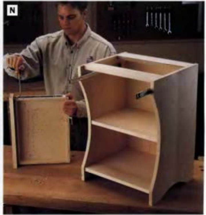
PHOTO N: install the full-extension metal drawer slides and hang the drawer in the cabinet carcass. Be sure there is an even overhang between the drawer face and the cabinet carcass.
