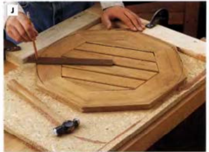
PHOTO J: Use a trammel to mark an 18-in.-dia. circle onto the underside of the tabletop, and cut it round with a band saw or jig saw.
