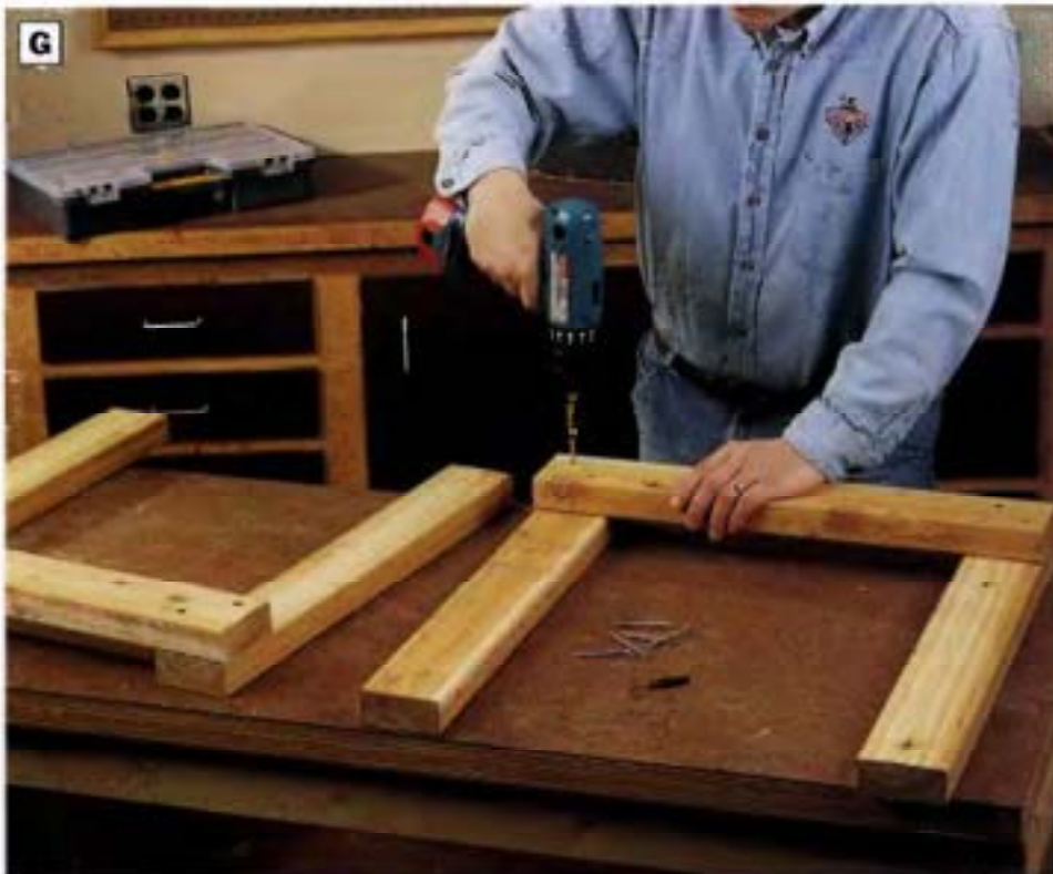
PHOTO G: Make the leg assemblies by fastening each arm support to a pair of legs. Drive pairs of 2½-in. countersunk deck screws through the arm supports and into each leg.
