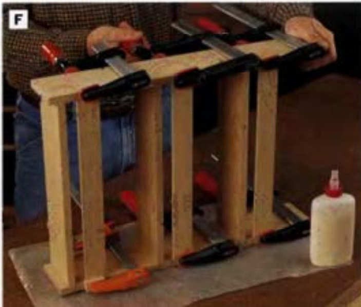
PHOTO F: Dry-fit the front rails in their notches in the sides. The rails should fit flush with the front edges of the sides. Once they do, glue and clamp the front rails in the notches.
