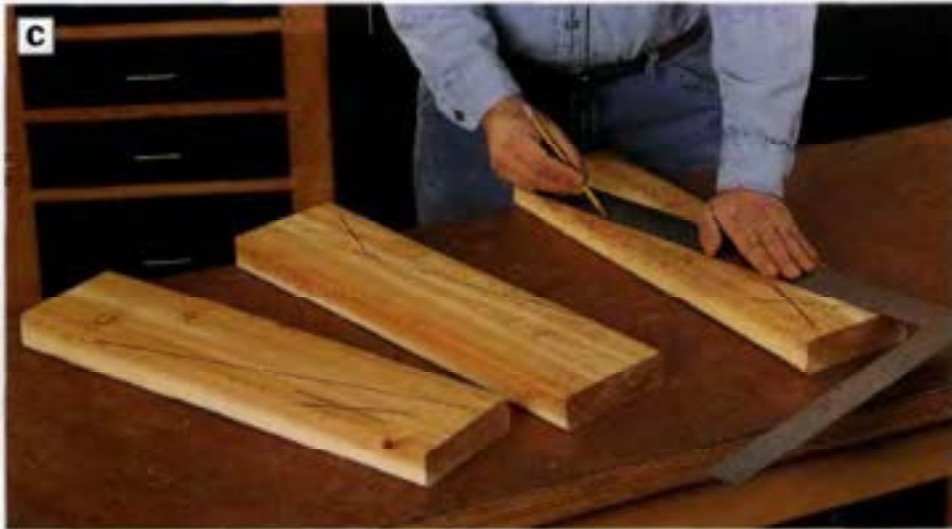
PHOTO C: Lay out the angled profile on the back support blanks with a straightedge.
