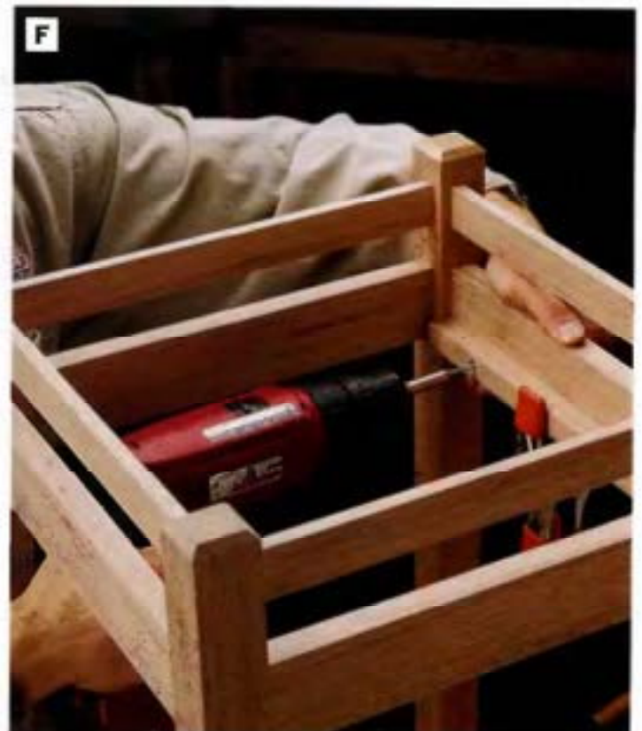
PHOTO F: Attach the tray cleats to the inside faces of the tray rails, using glue and #6 × 1¼-in. wood screws. The bottoms of the cleats should be flush with the bottom edges of the tray sides and should feature countersunk screw holes for attaching the tray bottom.
