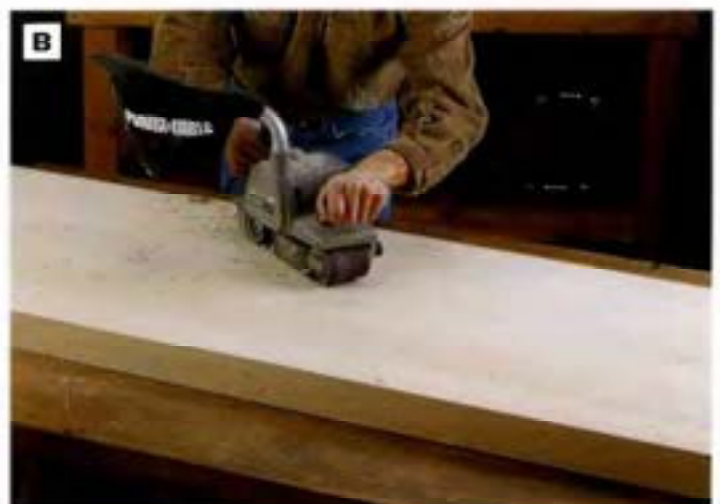
PHOTO B: Flatten the top and bottom surfaces of the benchtop, using a belt sander or a hand plane.
