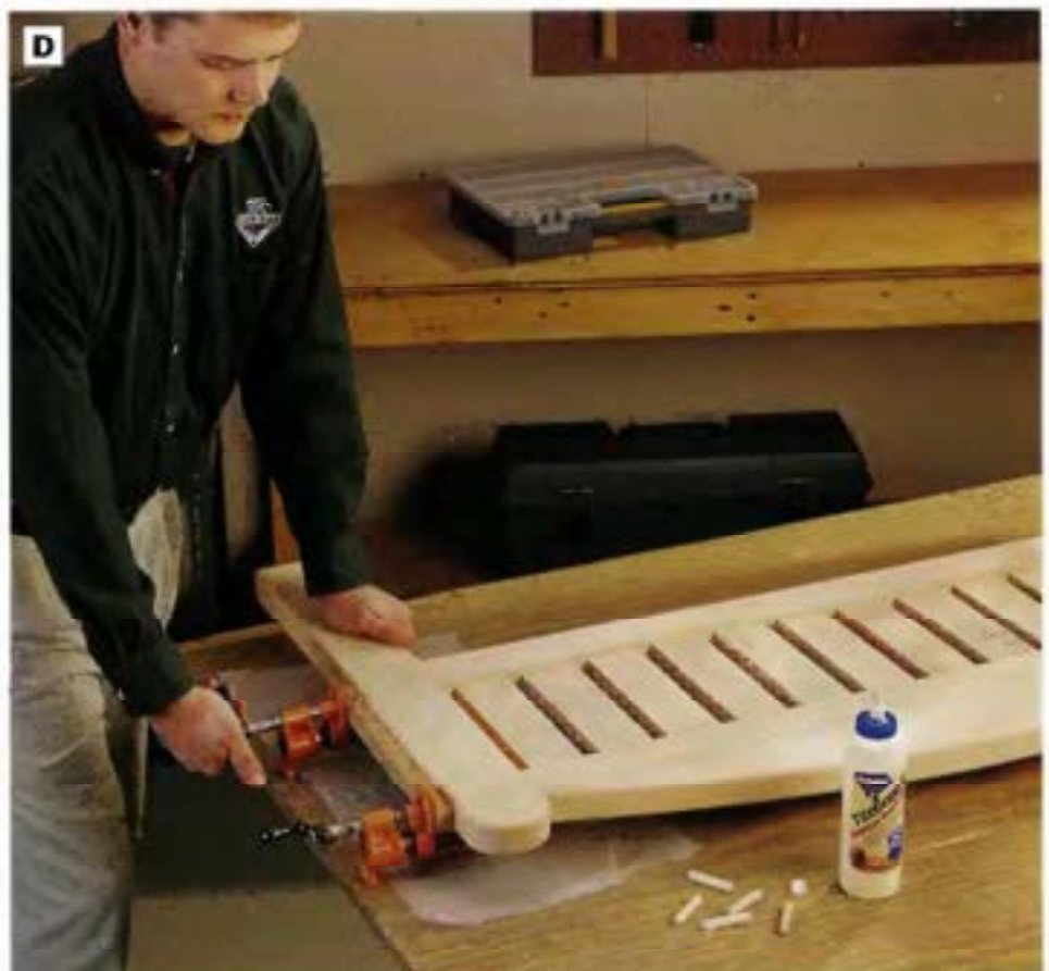
PHOTO D: Complete the back assembly by attaching the stiles to the back rails. Fasten the stiles to the ends of the rails with pairs of dowels and moisture-resistant wood glue.
