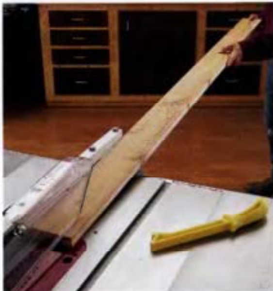
LONG BOARDS: When ripping long boards, tip the back edge of the board up so it is slightly higher than the saw table. Doing this will press the leading edge of the board firmly down on the saw table. Lower the back edge of the board as the cut progresses.
