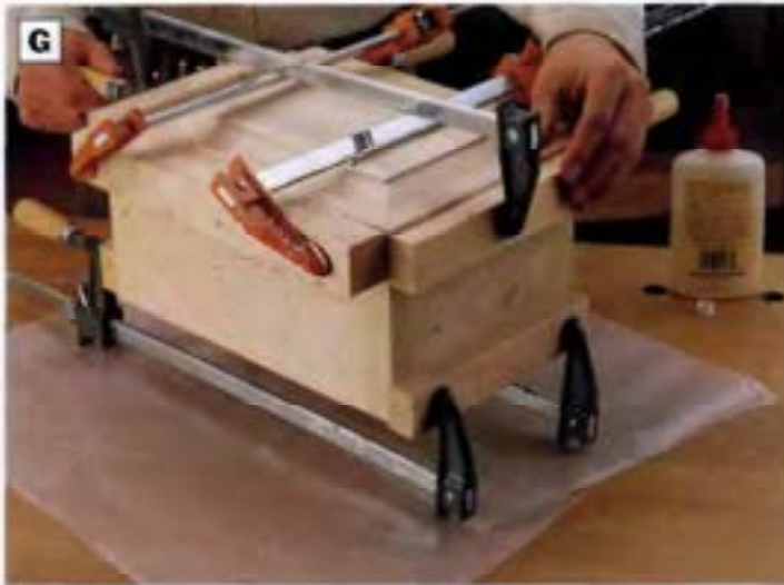
PHOTO G: Apply bar clamps across the box length and width to ensure tight miter joints. Wood cauls between the box and the clamp jaws will help distribute clamping pressure.
