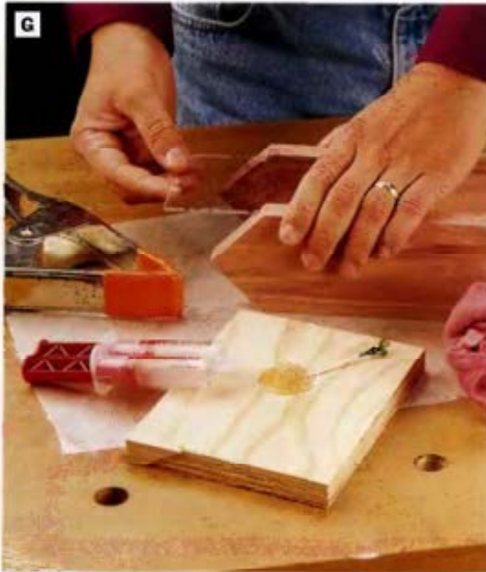
PHOTO G: Spread two-part epoxy into the grooves in the side panels, remove the protective film from the Plexiglas end pieces, and slide the end pieces into the grooves. The end pieces should stop \frac{3}{4} in. from the bottoms of the sides.
