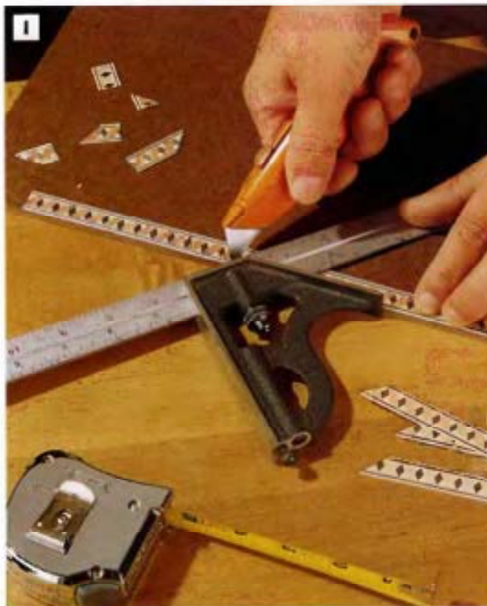
PHOTO I: Miter-cut the corners of the decorative inlay strips using the 45^\circ fence on a combination square and a sharp utility knife. Hold the knife as square to the inlay as you can when making the cuts, so the mitered joints will meet flush.
