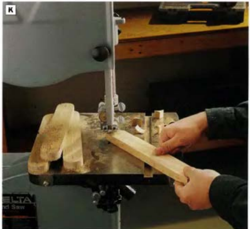
PHOTO K: Cut the four glider arms to shape on the band saw. Both ends of the arms receive \frac{7}{8} -in.-radius curves. Sand the cut edges smooth and round them over with a router if you wish.
