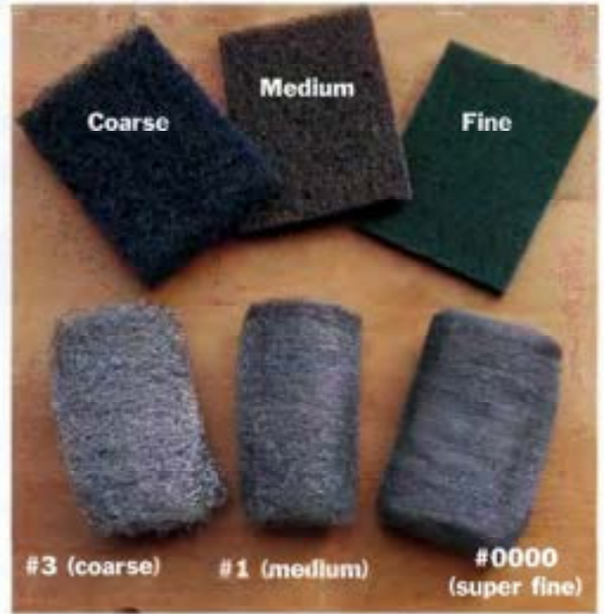
STEEL WOOL AND ABRASIVE PADS (synthetic steel wool) have many uses in the shop, from general cleanup to buffing to stripping old finishes.
