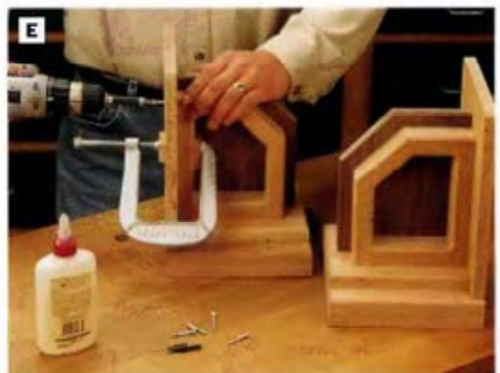
PHOTO E: Position the front plates on top of the bases, clamp them in place and attach them to the frame/divider assemblies with glue and four 1\frac{1}{4} -in. flathead wood screws.
