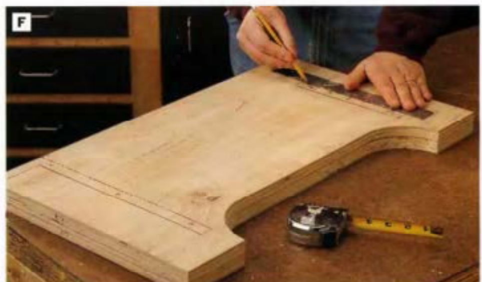
PHOTO F: Lay out the shelf and footrest positions on both sides of both desk legs. See the Side Elevation drawing, page 273, to position these parts.
