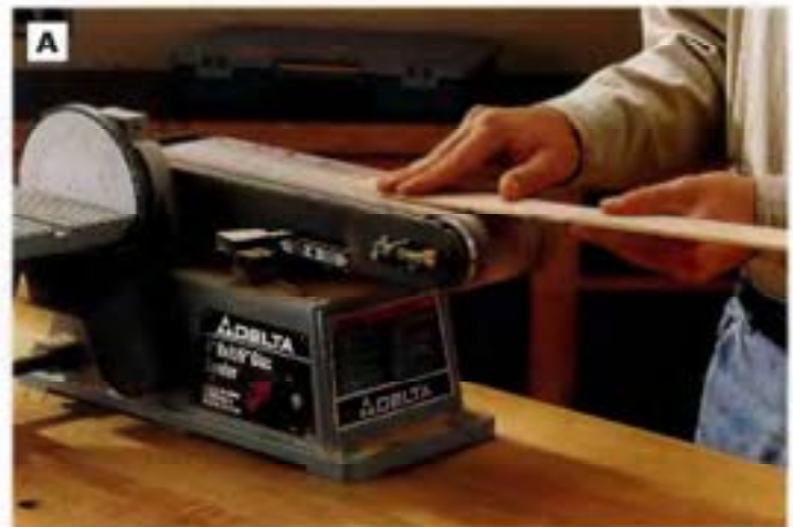
PHOTO A: The side pieces of both the lid and the box get tapered on one end to minimize the thickness of the overlap after they are bent to shape. Begin the taper about 2 in. in from one end of each part. A stationary belt sander works well for sanding these tapers.
