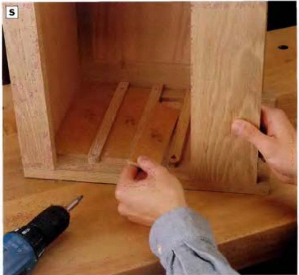
PHOTO S: Mount the drawer slides using spacers to maintain even placement. After the slides are in place, remove the spacers.
