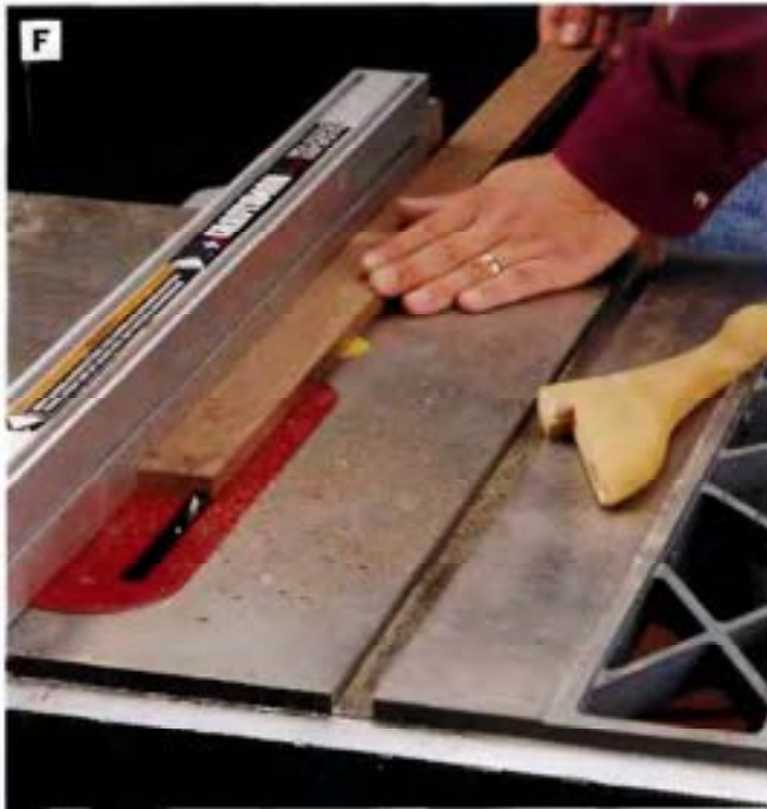
PHOTO F: Cut the \frac{1}{8} -in.-wide groove for the box bottom using a dado blade in the table saw. Then install a \frac{1}{8} -in.-kerfed blade in the saw and cut a groove for the sliding lid along the opposite long edge of the workpiece. Cutting these grooves now allows you to work more safely with a long workpiece and ensures that the grooves will align perfectly when you assemble the box later.
