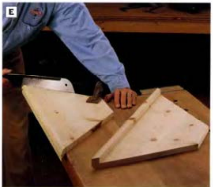
PHOTO E: Clamp the fixed shelves to your workbench and trim the profiled shelf edging to match the angled ends of the shelves. We used a fine-toothed Japanese-style pull saw to make the cuts.
