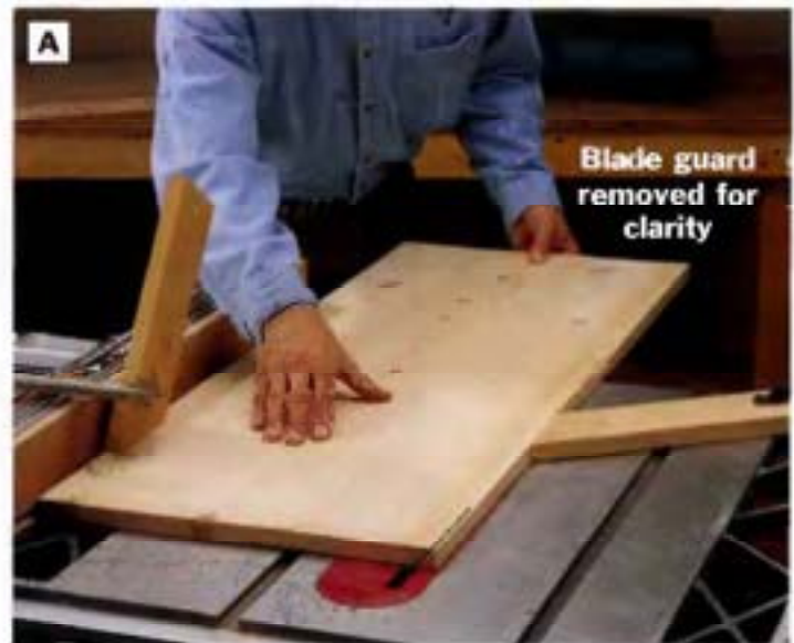
PHOTO A: Bevel-rip the glued-up panels on both edges to make the cabinet sides. The 45° bevels should be parallel. Clamp featherboards to the saw table and fence to hold the panels securely as you cut.
