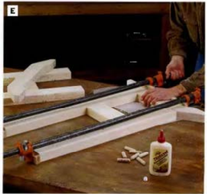
PHOTO E: Use pipe clamps to draw the feet tightly against the bottoms of the legs.
