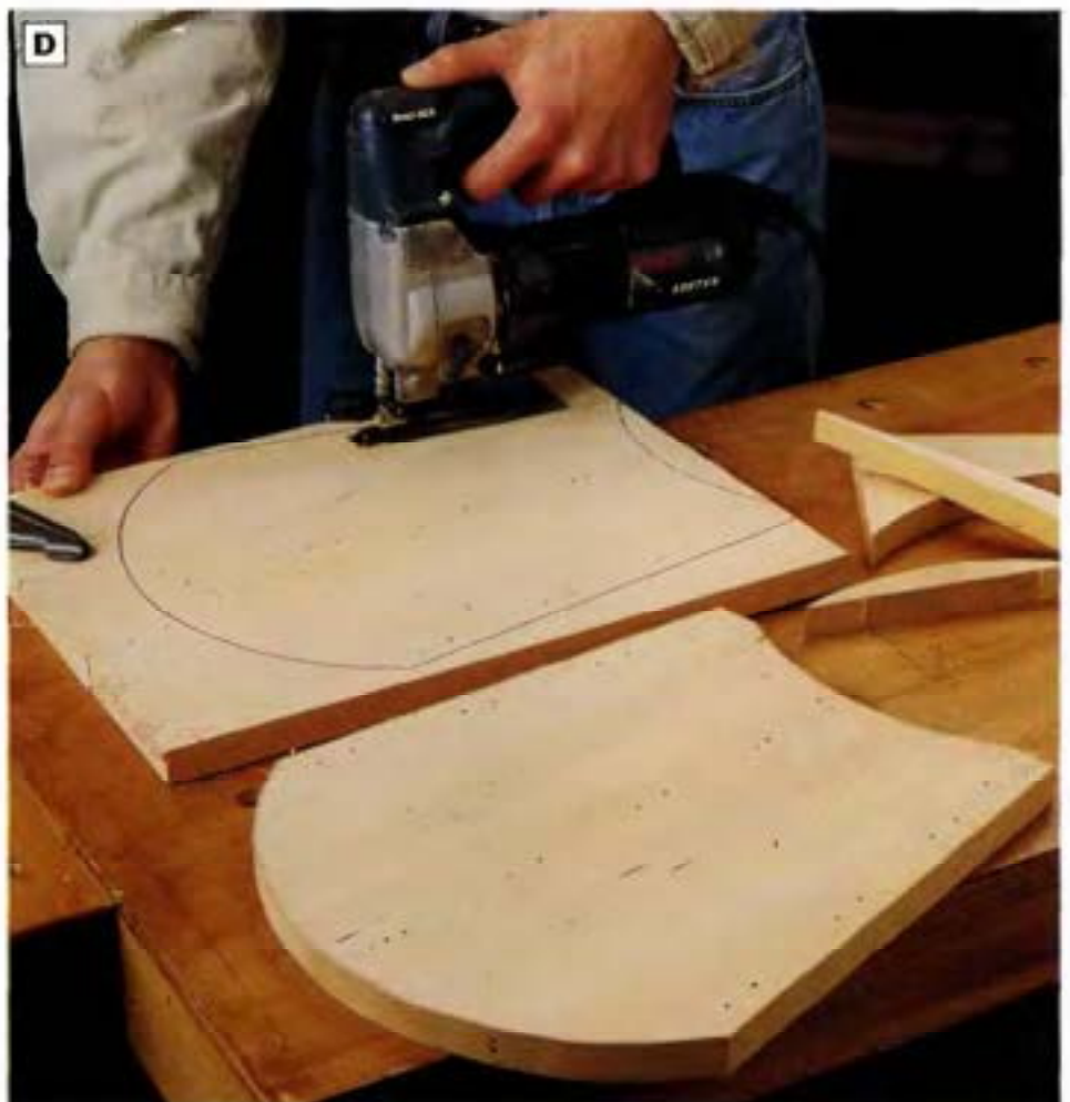
PHOTO D: Cut out the end shapes. We used a jig saw, but you could use a band saw or scroll saw instead. Cut along the waste sides of the cutting lines, then smooth the cuts with a file or by sanding with medium-grit sandpaper.
