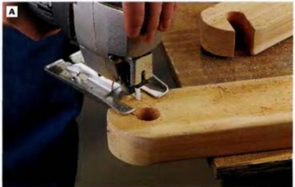
PHOTO A: Cut notches in the seat rails for back rest and foot rest dowels by boring 1-in.-dia. holes in the rails first, then cutting through the rails to the holes to form the notches. The foot rest notch (shown) is angled 45^\circ on the seat rail, while the back rest notches are perpendicular.
