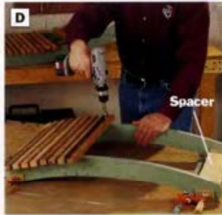
PHOTO D: When installing the back and seat slats to the supports, clamp scrap spacers between the supports to keep them aligned.
