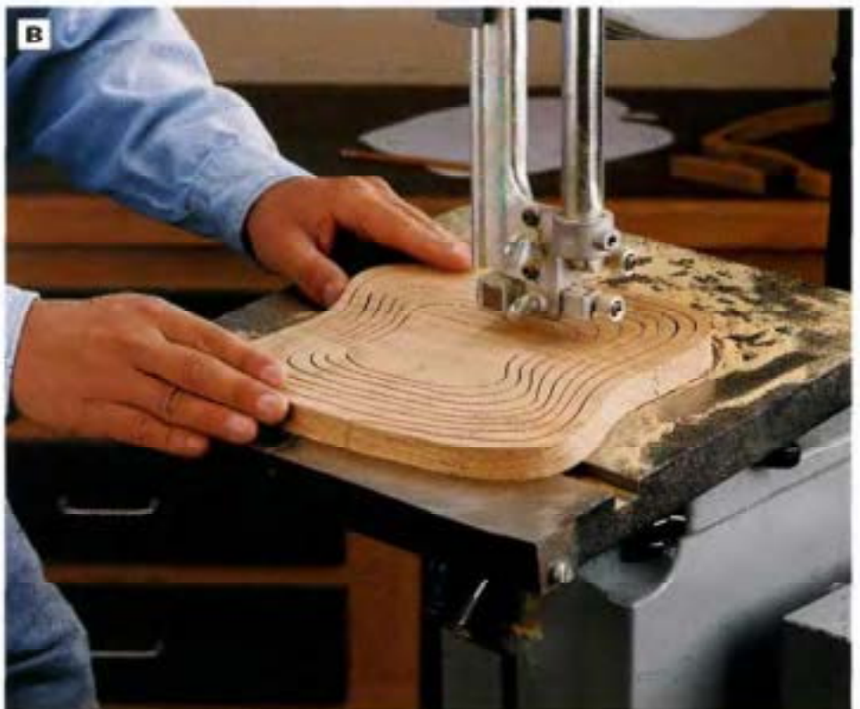
PHOTO B: Tilt the saw table to 3° and begin the spiral cut, orienting the workpiece so the blade tilts in toward the center of the basket throughout the cut. Take your time making this spiraling cut, following your layout lines closely. Try to complete the spirals in one continuous cut.
