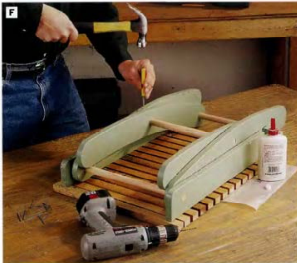
PHOTO F: Install the inner legs between the outer legs, and insert the leg pivot dowel through the center dowel holes in the legs. Cut and insert the table lock dowel through the inner legs. Pin the table lock dowel to the inner legs and the leg pivot dowel to the outer legs with finish nails.
