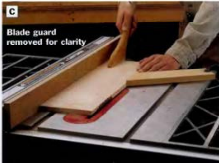
PHOTO C: Cut a 15° bevel into the top edges of the two resawn box boards. Use a featherboard and pushstick for accuracy and safety.
