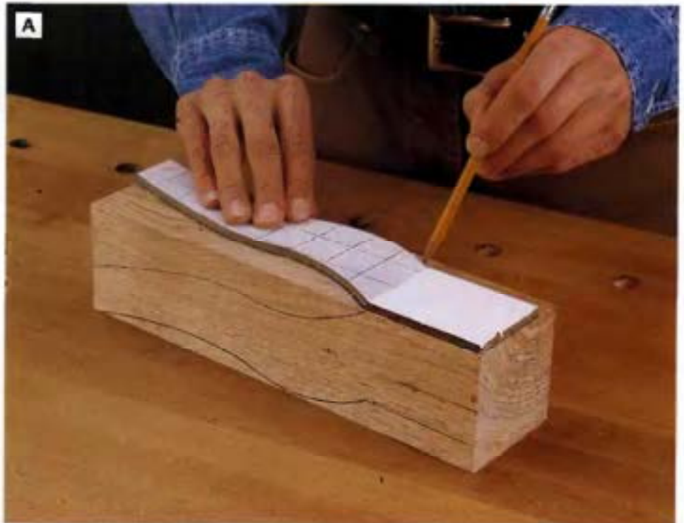
PHOTO A: Create a leg template from scrap hardboard. Trace the leg shape onto one face of each leg blank, holding it flush against the inside top corner of the wood. Then trace the leg profile onto the adjacent side of the blank.
