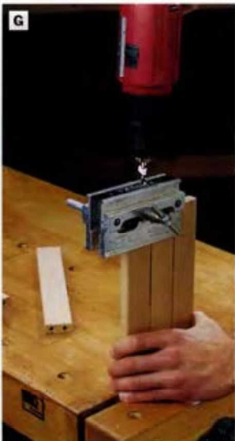
PHOTO G: Use a doweling jig to drill centered dowel holes in the ends of the rails and handle. Clamp rails together edge-to-edge to provide more surface area for the jig.
