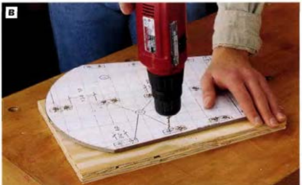
PHOTO B: Drill small locator holes through the side template, at the centerpoints shown for each dowel location. Use scrap plywood underneath to prevent drill bit tear-out.
