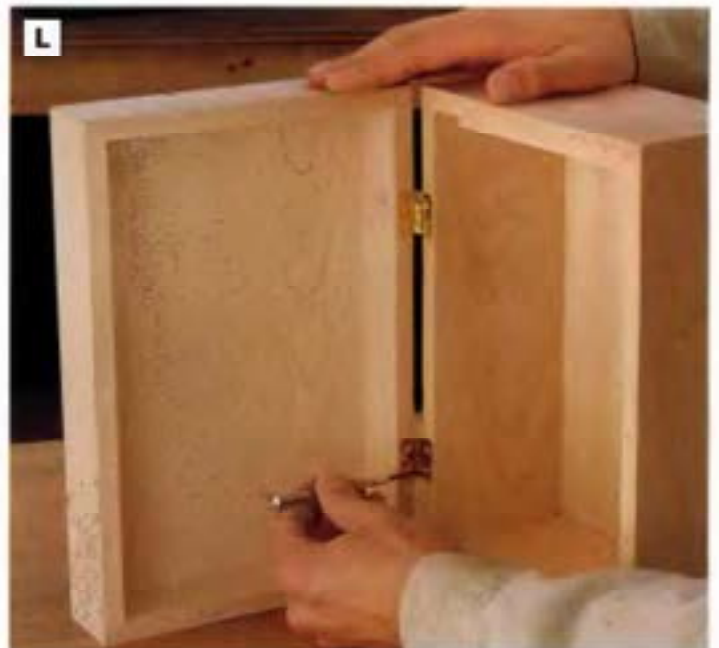
PHOTO L: Measure and cut the hinge mortises with a wood chisel, then install the brass jewelry box hinges to attach the lid to the box.
