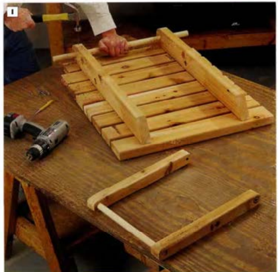
PHOTO I: Tack the back rest dowel in place on the back rest rails with #6d galvanized finish nails. Drive the nails through the rails and into the dowels. To keep the dowels from splitting, drill a pilot hole for the nails first.
