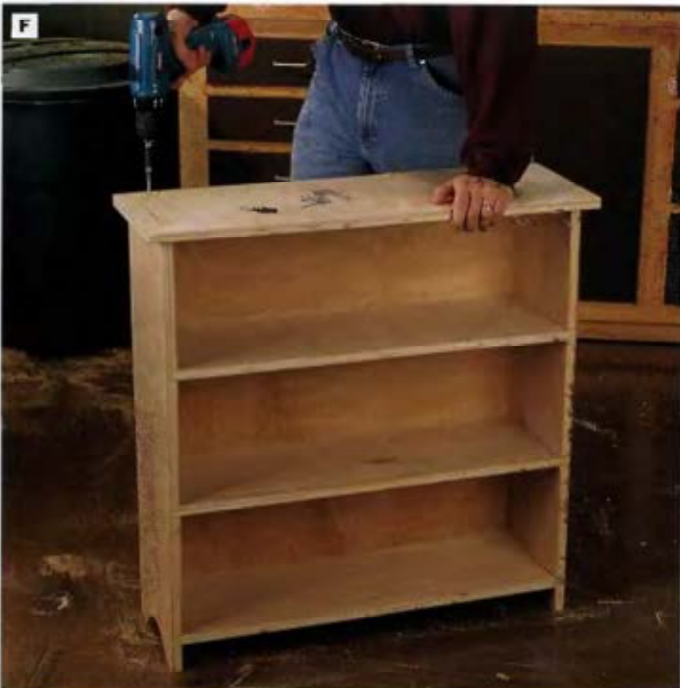
PHOTO F: Position the top panel on the bookcase and fasten it with 2-in. drywall screws driven into countersunk pilot holes.
