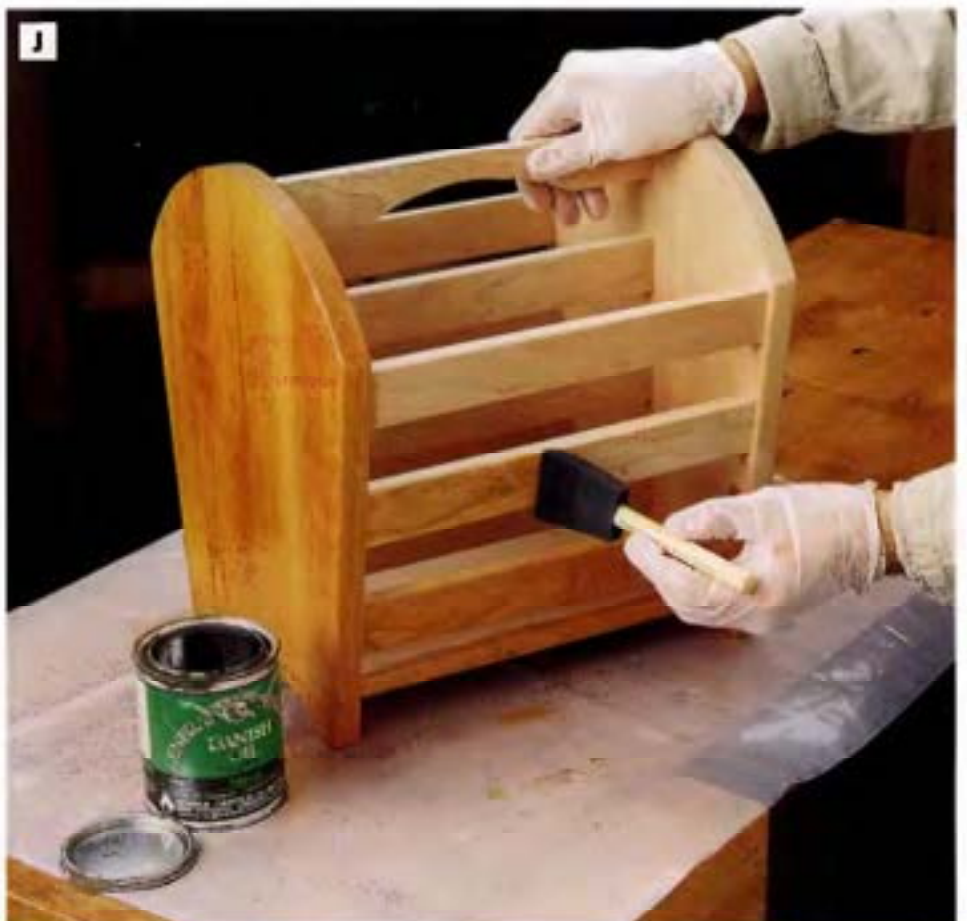
PHOTO J: Because of all the flat, narrow surfaces that are easy to access, a brush-on finish is a good choice for this magazine rack. We used three coats of Danish oil for an even, satiny finish.
