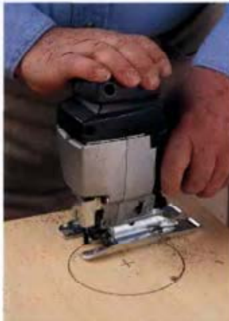
THE VERSATILE JIG SAW (also called a saber saw) is capable of making any cut. It excels at cutting curves and making interior cutouts.
