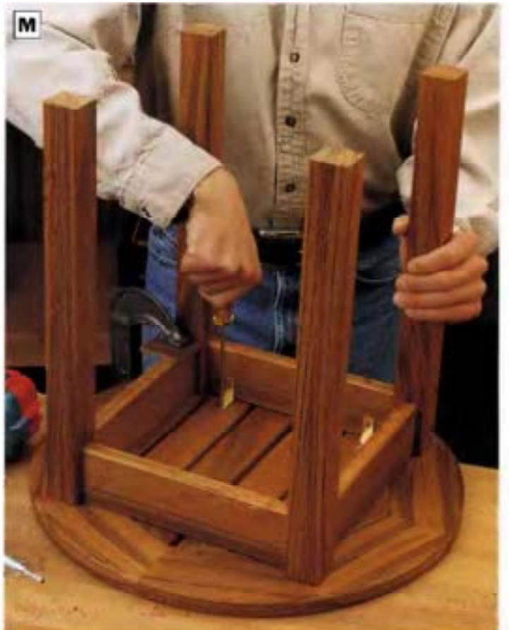
PHOTO M: Attach the tabletop to the rails and legs using brass L-brackets. Drill pilot holes before driving the screws.
