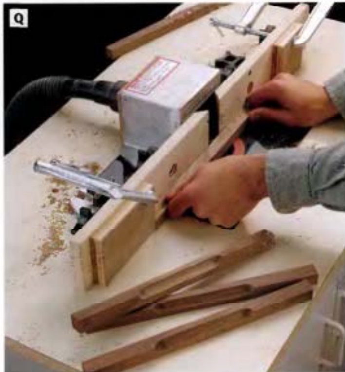
PHOTO Q: With the bit spinning, feed the workpiece up against the fence, making sure it contacts the start block. Then, feed it toward the stopblock until the cut is finished.
