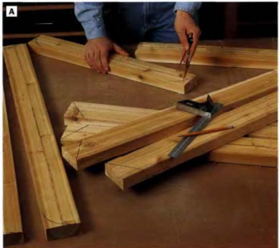
PHOTO A: Lay out the legs and stringers. Scribe the curved end of the legs and the curves on the stringers with a compass, set to the radii given in the technical drawings on page 300.
