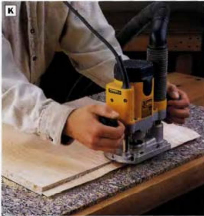
PHOTO K: Trim overhanging veneer with a router and a flush-trimming bit so the edges are flush with the tabletop.
