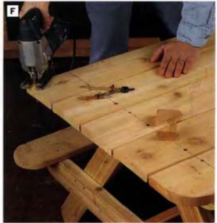
PHOTO F: Mark a 2\frac{3}{4} -in. radius on each of the four corners of the tabletop, and trim the corners with a jig saw.
