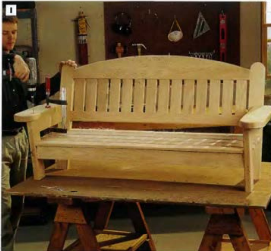
PHOTO I: Cut the arm rests to shape, ease the edges with a router and roundover bit, then clamp them on top of the arm supports. Attach the rests to the supports with countersunk screws.
