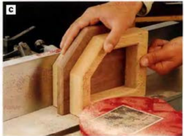
PHOTO C: Flatten the long edges and bottom ends of the frame/divider assemblies on the jointer or sander. The purpose here is to produce flat, even surfaces to attach to the base caps and front plates.
