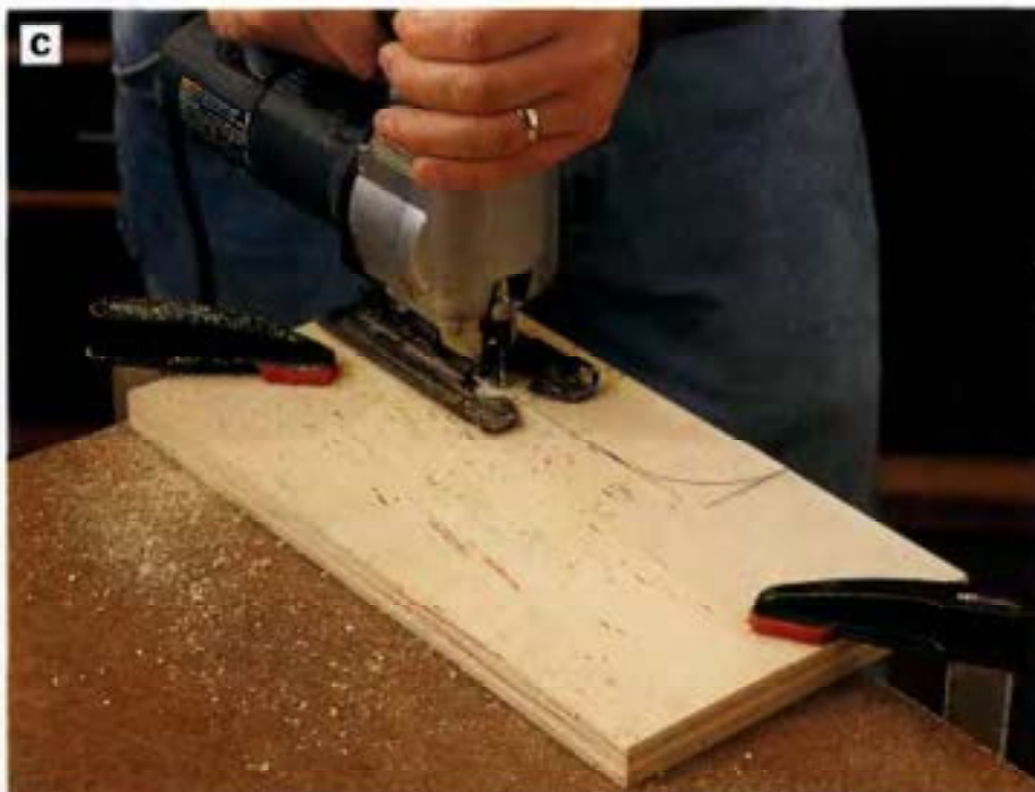
PHOTO C: Clamp each bench leg to your workbench and cut to shape with a jig saw. Be sure your clamps don't interfere with the path of the saw.
