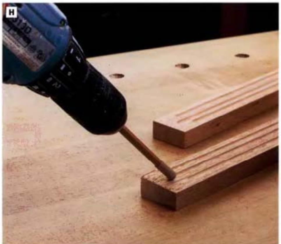
PHOTO H: Use a homemade flute sander to remove any burn marks and smooth the ends of the flutes. Wrap adhesive-backed sandpaper around the eraser of a pencil section chucked in your drill, and run the drill at low speed.
