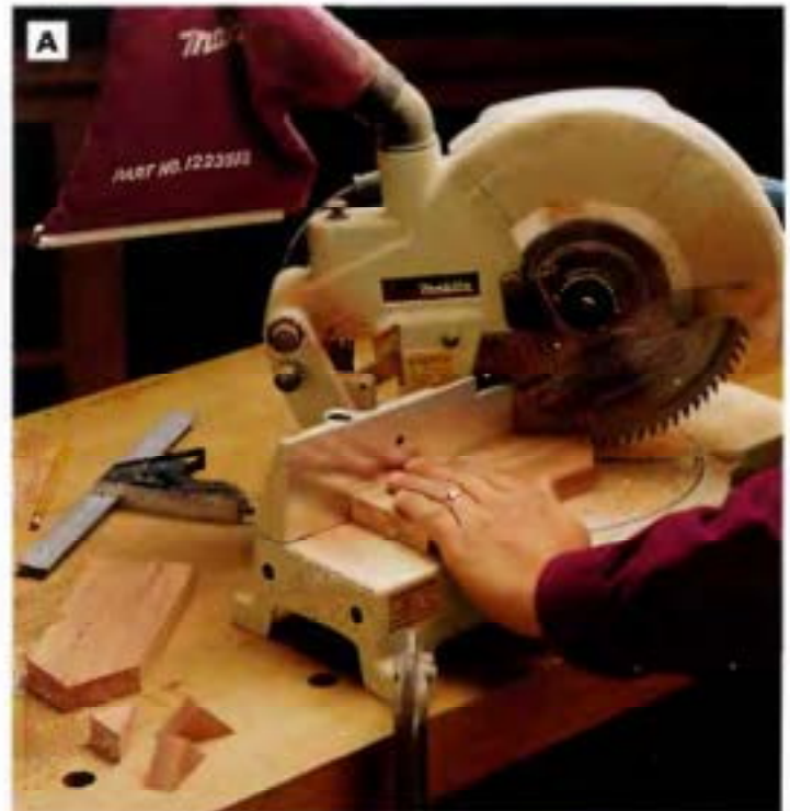
PHOTO A: Trim the gable ends of the sides on a power miter saw with the blade swiveled to 45°. Center the gable peaks across the width of the workpieces.
