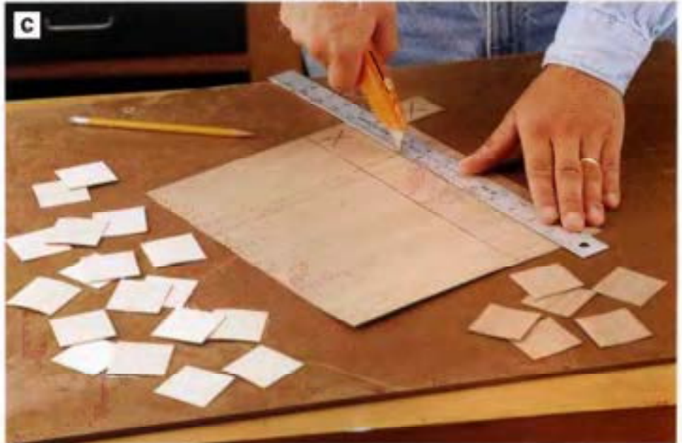
PHOTO C: Lay out and cut the chessboard squares from walnut and maple self-stick veneer. Make 32 of each, using a straightedge and utility knife to cut them out. Hold the blade vertically as you cut so that the edges will be square and fit tightly together.
