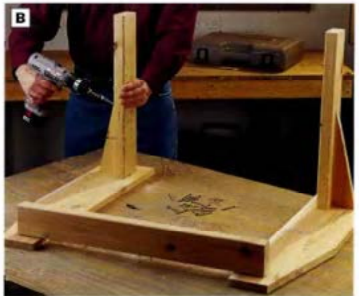
PHOTO B: Attach the back support, front legs and arm braces to the arm workpieces with 2-in. galvanized screws.
