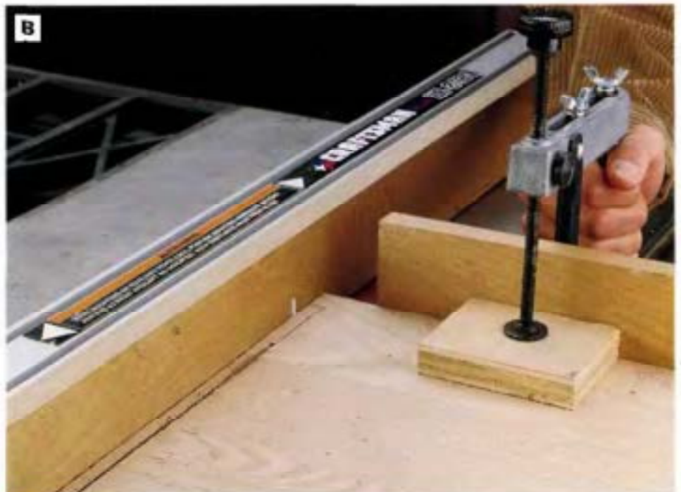
PHOTO B: Cut notches in the ends of the upper cabinet's top and bottom panels. Stop the cuts before the blade cuts past the end line of the cuts, and finish the cuts with a hand saw or jig saw. The notches create a \frac{3}{8} \times \frac{3}{4} -in. tab that fits over the front edge the side panel on the upper cabinet, creating a recess below for the cabinet door frames.
