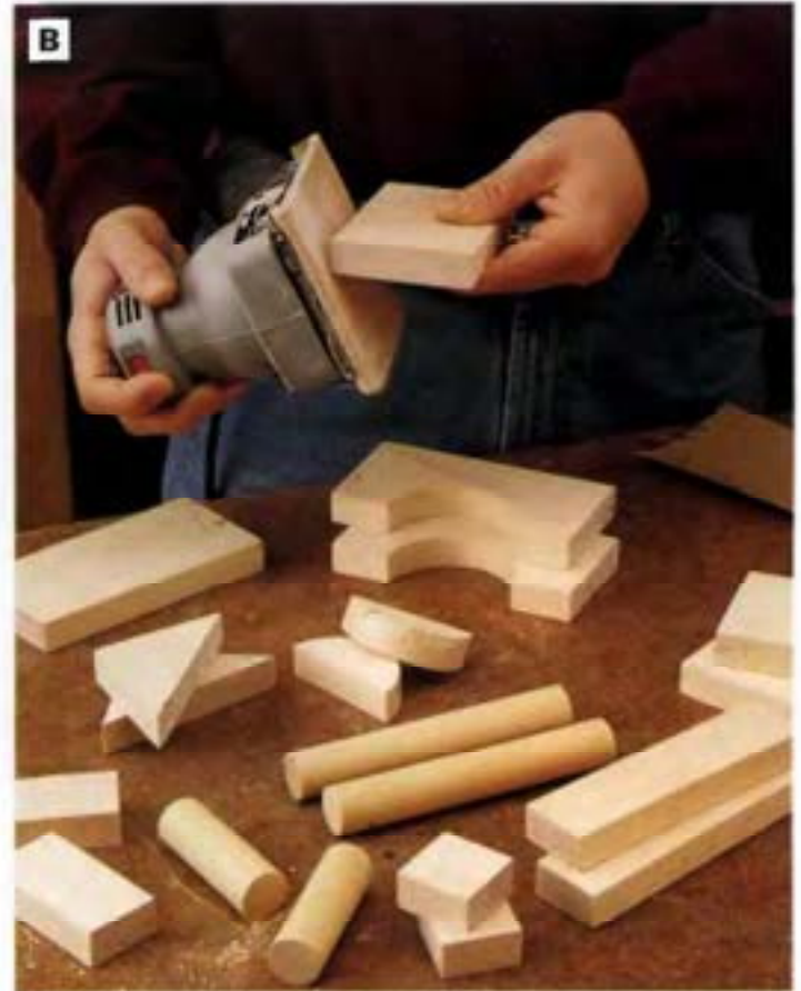
PHOTO B: Sand the blocks thoroughly to remove all sharp corners, edges and any splinters.
