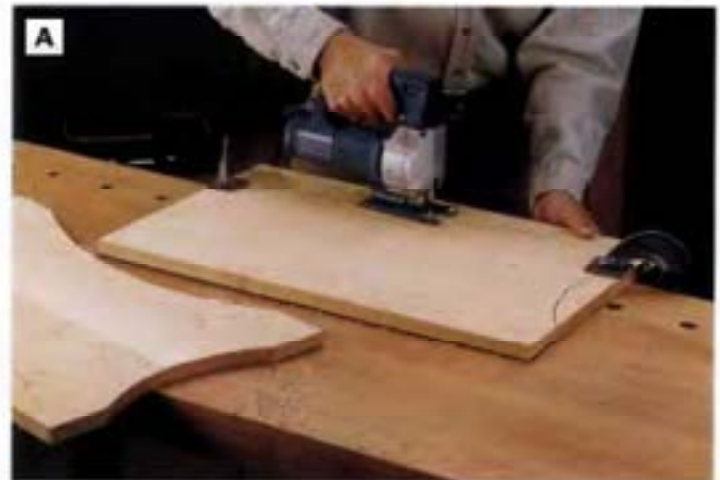
PHOTO A: Lay out curves on the sides, and cut them out with a jig saw or a band saw.
