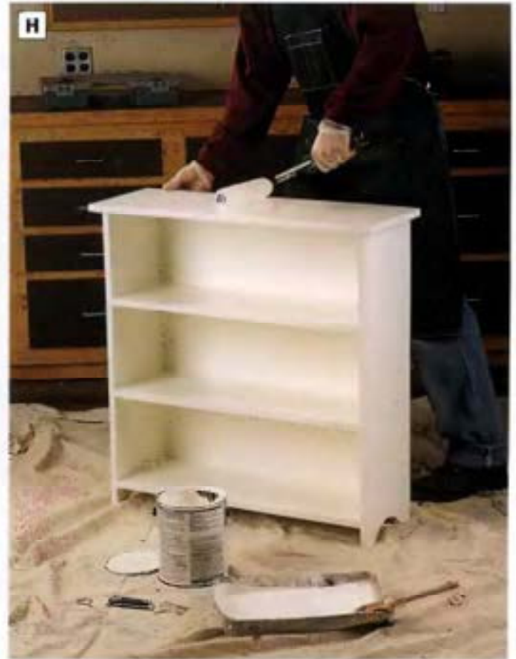
PHOTO H: Roll or brush on a coat of primer to all exposed surfaces, followed by two coats of paint.
