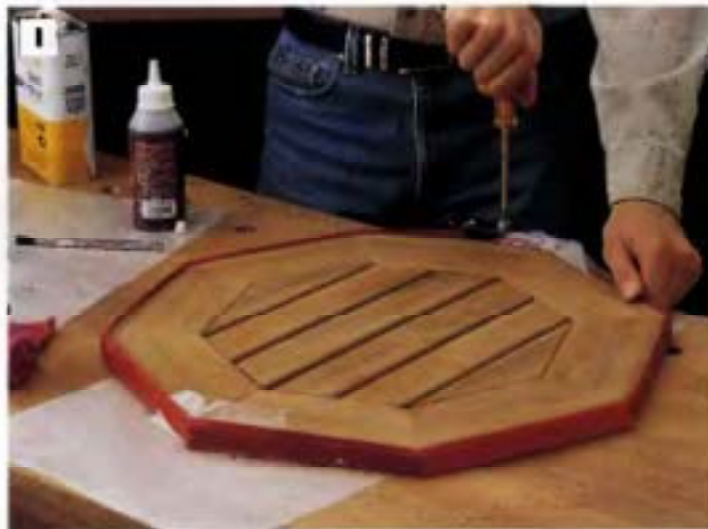
PHOTO I: Glue and clamp the two halves of the tabletop rail assembly together with polyurethane glue and a strap clamp. Cover the glued corners with wax paper. Nail, rather than glue, the slats in place.
