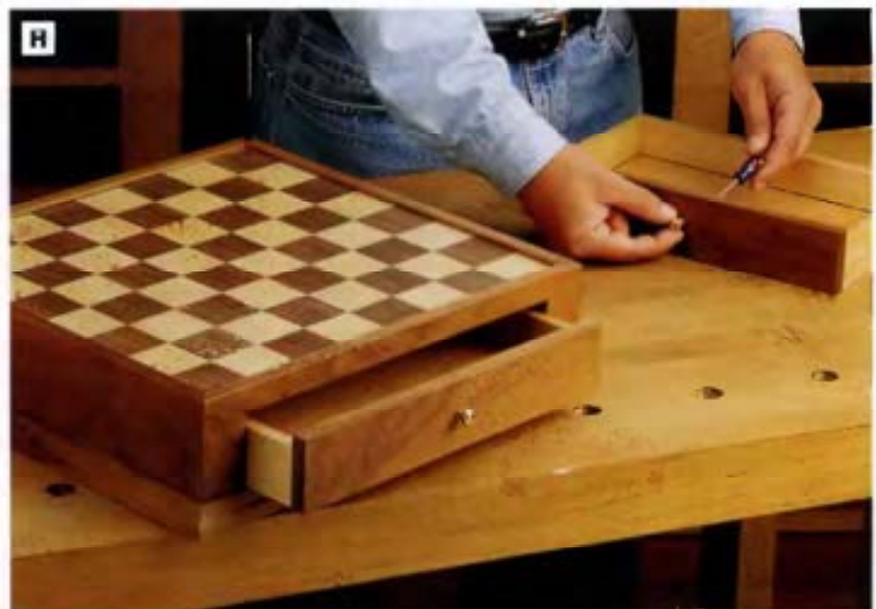
PHOTO H: After applying three coats of satin polyurethane, install the knobs on each drawer. Although we don't show it here, you may also want to add catches or turnbuckles for holding the drawers closed for transport.
