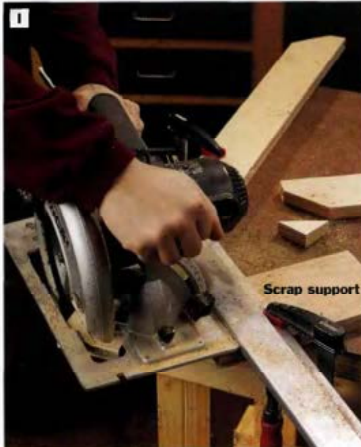
PHOTO I: Mark the angled ends of the runners and cut the corners with a circular saw. Support your straightedge from beneath with a wood scrap clamped to the workbench.
