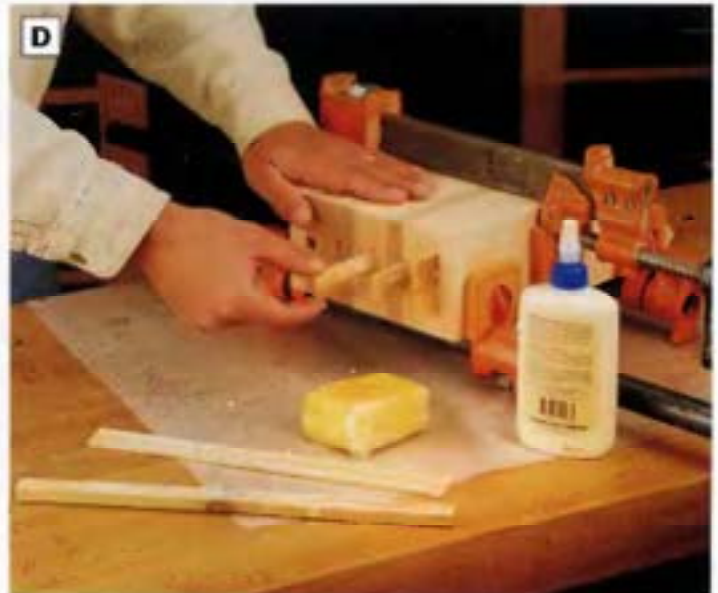
PHOTO D: After your clamps have squeezed the excess glue from the assembly, but before the glue starts to set, remove the wax-coated filler strips in the knife slots. Once the glue dries, sand the block smooth.
