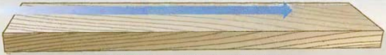
Straight grain: Plane following the upward grain slope
