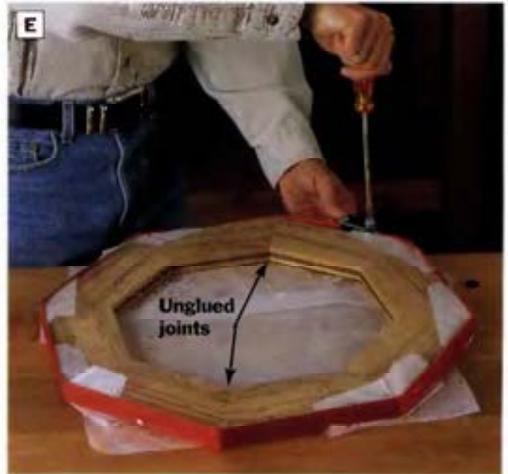
PHOTO E: Clamp the top rail assembly with a strap clamp, leaving two opposite joints unglued. Use wax paper around the glued corners to keep the strap from bonding to the wood.
