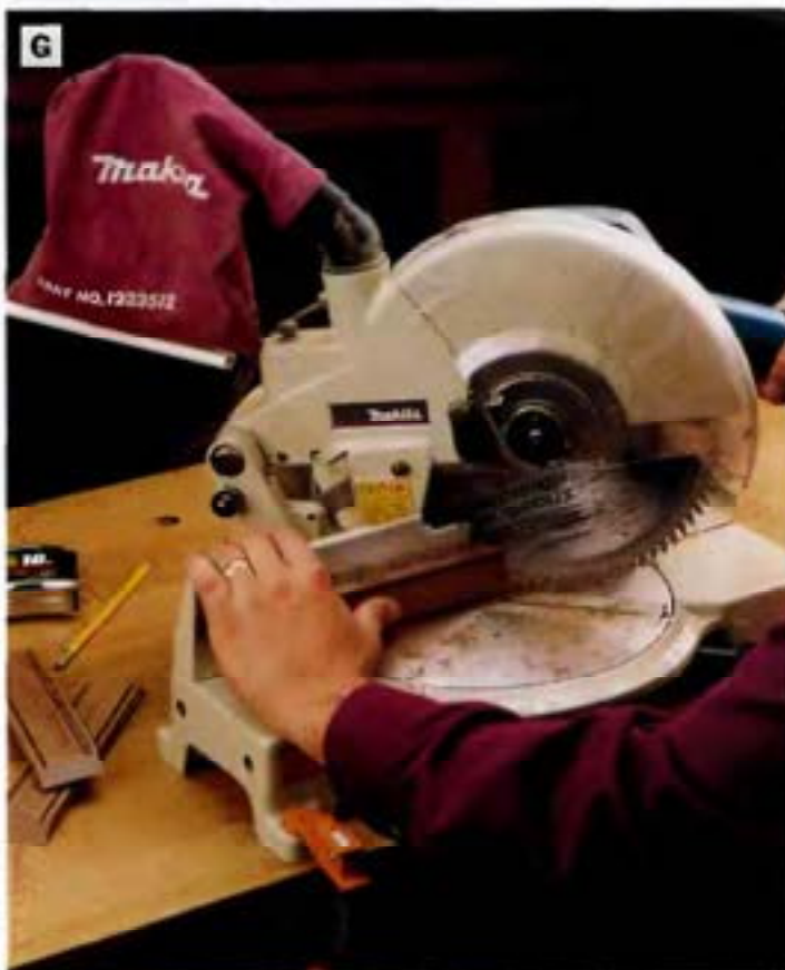
PHOTO G: Cut the box sides and ends to length. We set a power miter saw to 45^\circ so that the parts would be both cut to length and also mitered for assembly. Accuracy is especially critical if you perform both of these operations in one step.
