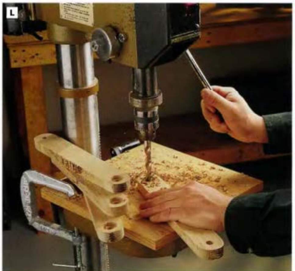
PHOTO L: Bore \frac{3}{16} -in.-deep, 1-in.-dia. counterbores on both ends of the glider arms. Notice that the counterbores are on opposite faces of the arms. Then drill a \frac{1}{2} -in.-dia. hole through the center of the counterbores all the way through the arms, to accommodate the pivot hinges.
