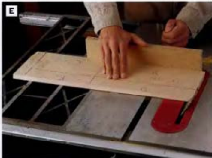
PHOTO E: Cut the sides to length on the table saw, mitering the ends at the same time. Use a miter gauge set to exactly 90° to feed the stock through the blade.
