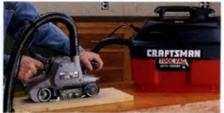
A TOOL VAC is a relatively new entry in the dust collection field. It's similar to a shop vac in size and power. Tools are connected to the power source through a receptacle mounted on the tool vac. This allows the vac to shut on and off automatically as the tool is used.
