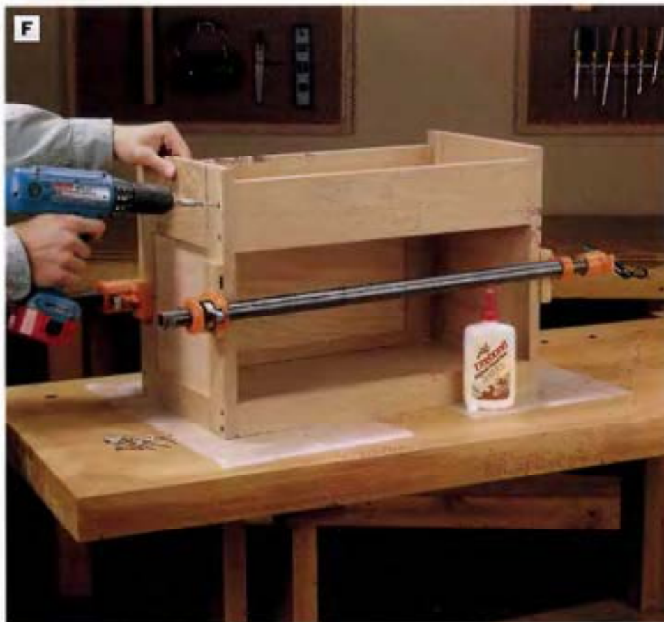
PHOTO F: Glue up the frame-and-panel assemblies and the chest bottoms to create the chest carcass. Reinforce the joints by driving screws through the side panels and into the ends of the front and back rails. Counterbore the pilot holes to accept \frac{3}{8} -in.-dia. wood plugs.
