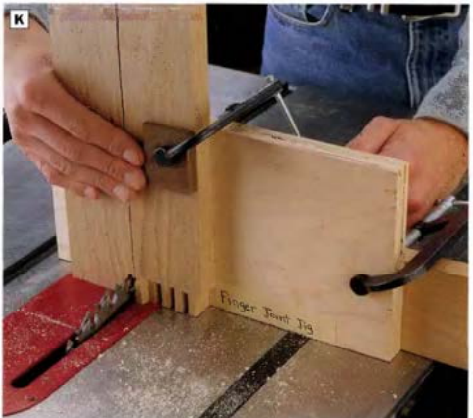
PHOTO K: For boards that start with a slot, not a pin, use the mating board as a guide for cutting the initial slot. The end slot on the cut board fits over the pin spacer strip, with the outer pin on the workpiece fitting between the strip and the saw blade.
