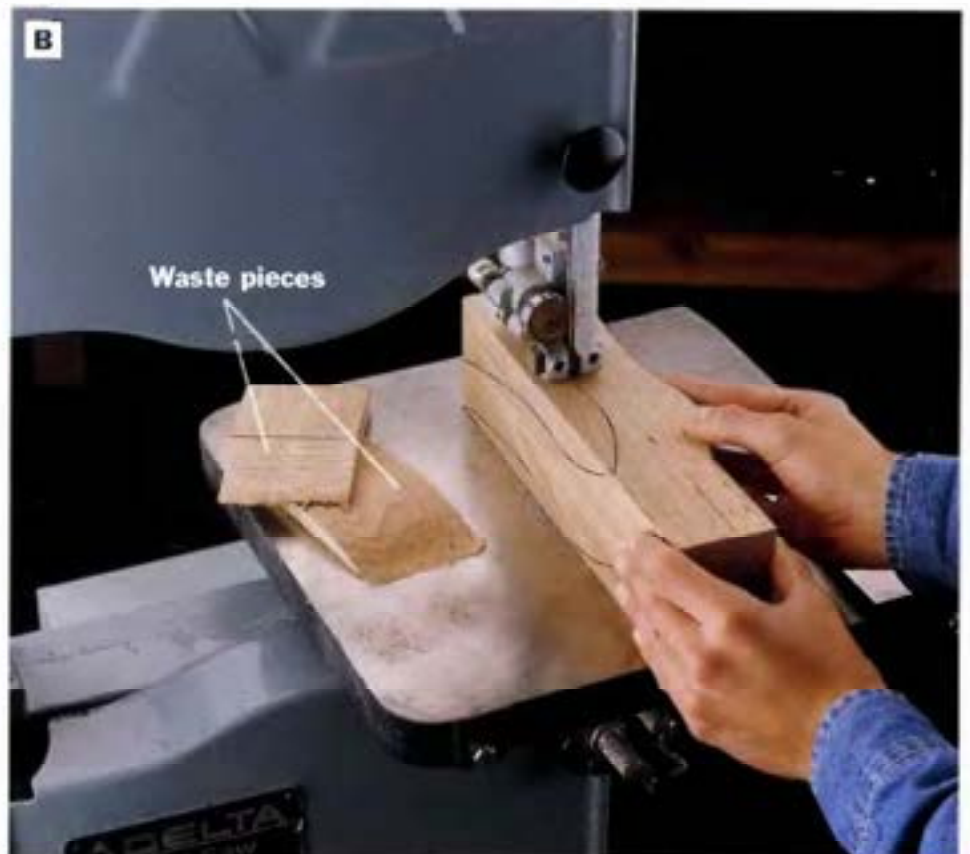
PHOTO B: To cut the legs to shape, start by cutting out the profile on one face of each leg blank on the band saw. Save the waste pieces, and try to cut them out in single sections.
