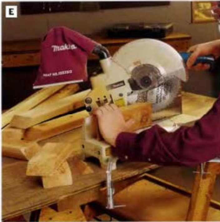
PHOTO E: Miter-cut the ends of the leg braces and table aprons to 45°. The safest way to make these cuts, particularly on the short leg braces, is to use a power miter saw or table saw rather than a circular saw.
