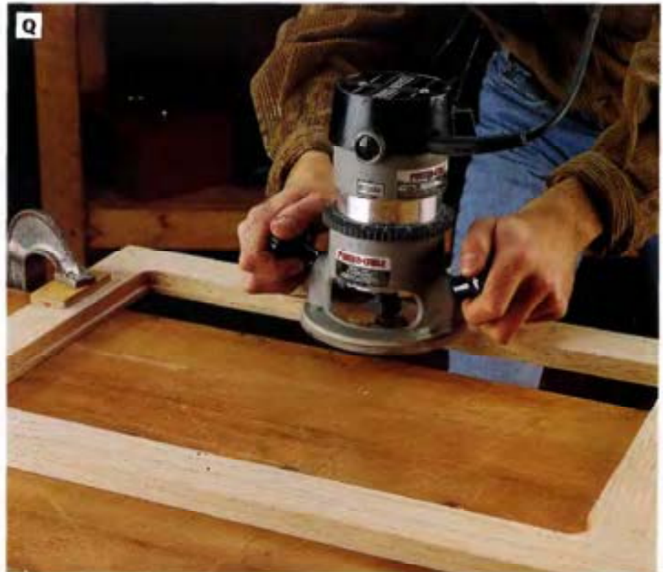
PHOTO Q: Rout a \frac{1}{4} \times \frac{1}{2} -in.-deep rabbet recess around the perimeter of each opening in the upper cabinet doors. Use a \frac{1}{4} -in. piloted rabbet bit (See page 137) to make the cuts. Square off the rounded corners left by the router bit, using a sharp chisel. To keep the wood from tearing, score along the chisel lines with a sharp knife before squaring the corners.
