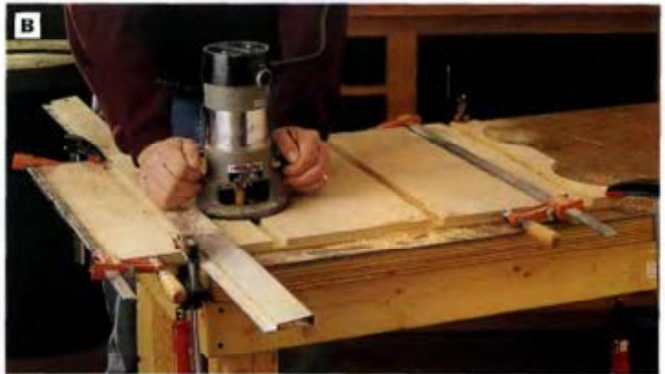
PHOTO B: Clamp the sides together side by side, lay out the shelf dado locations and gang-rout the dados across both sides. Clamp a straightedge across the side workpieces to guide the router cuts.
