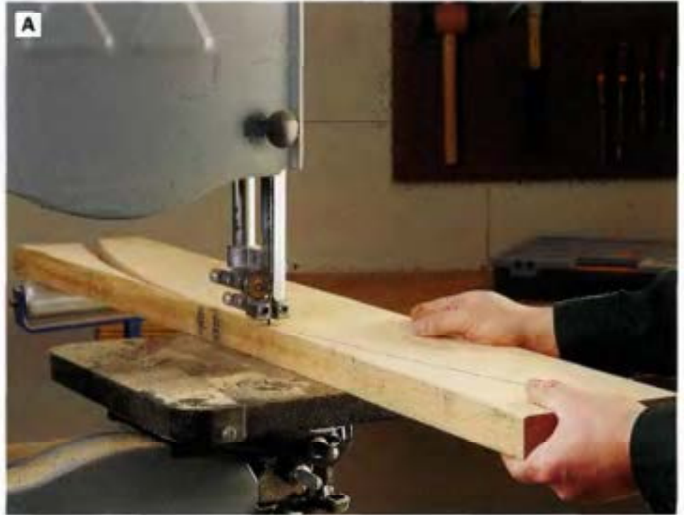
PHOTO A: Cut the profile on the upper back rail to shape on the band saw. Save the curved cut-off pieces to use as cauls when you clamp the back rails and slats together later.
