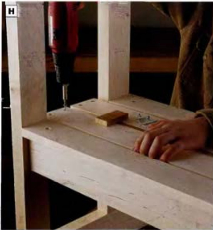
PHOTO H: Screw the inner and outer slats to the stretchers and cross braces to create a storage shelf.
