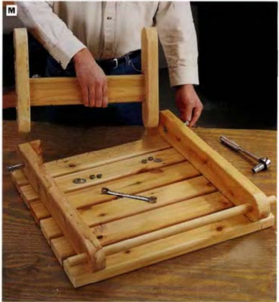
PHOTO M: Attach the foot rest stretcher to the legs with 2½-in. deck screws, then join the leg assembly to the foot rest with bolts, washers and double nuts.
