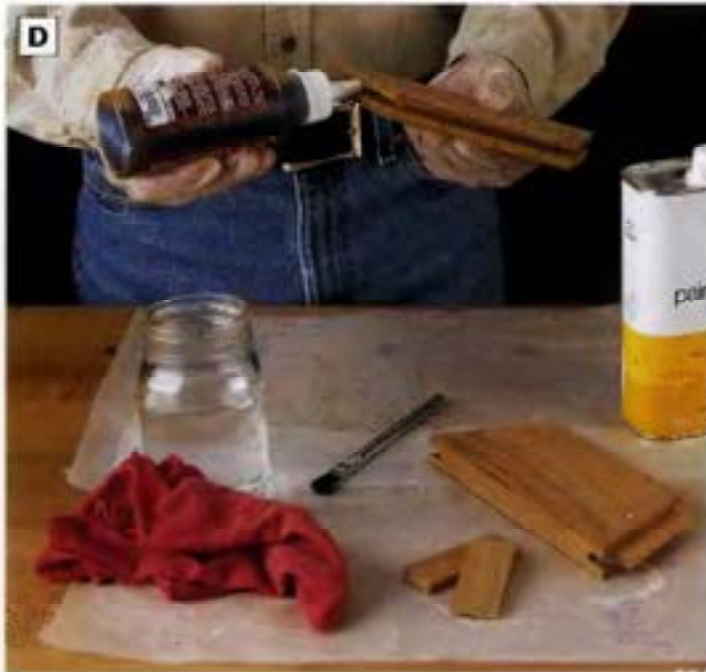
PHOTO D: Glue the splines into the tabletop rail end grooves. Wipe the mating parts first with mineral spirits to remove the natural oils in the wood. Spread the glue evenly with a glue brush. Wear latex gloves and have mineral spirits and a rag handy to wipe up squeeze-out.
