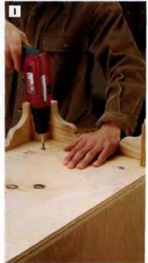
PHOTO I: Attach the base to the underside of the lower cabinet with screws and washers. The screw slots in the platform allow the screws to move as the wood moves.
