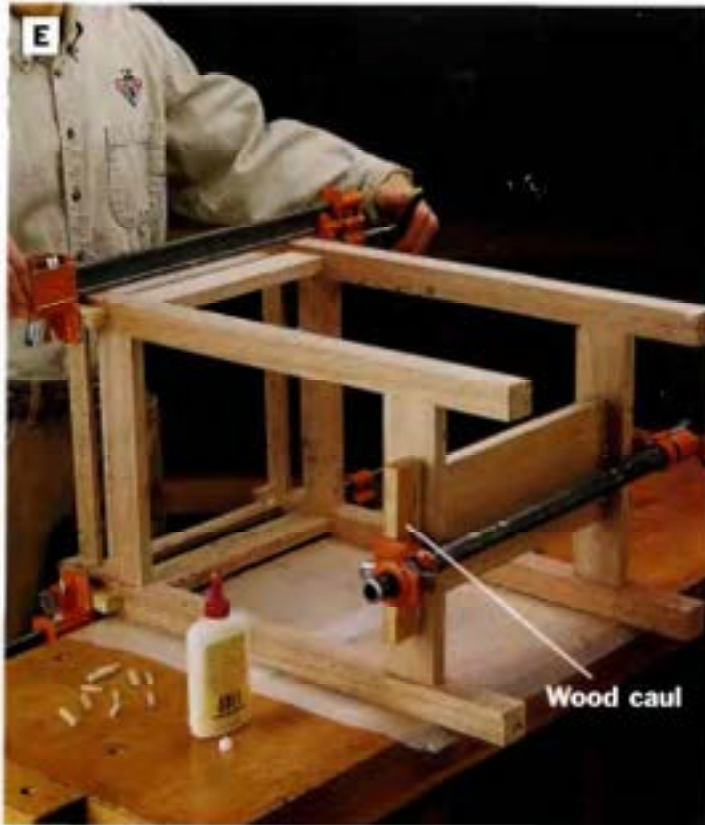
PHOTO E: Glue up the frame base for the plant stand. Slip wood cauls between the heads of the bar or pipe clamps and the plant stand. Position the cauls so they distribute the clamping pressure evenly across multiple joints, if possible.
