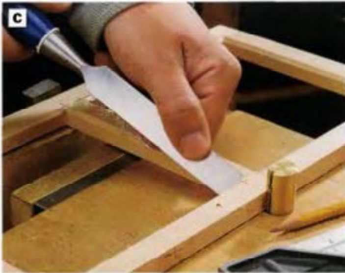
PHOTO C: Square off the inside chamfered corners of the face frame with a chisel. Lay out these corners first with a pencil and square, then pare up to your layout lines.
