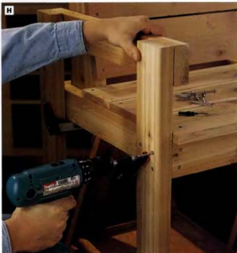
PHOTO H: Position and clamp the leg assemblies to the ends of the bench seat and attach the parts with screws. The arm supports should face inward.
