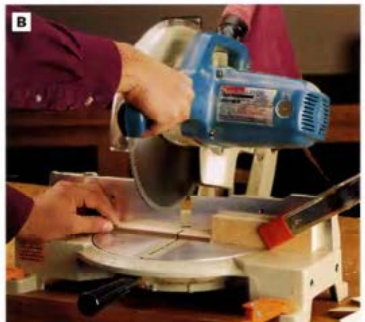
PHOTO B: Crosscut the laminated strips into individual domino tiles using a stopblock clamped to the fence of a power miter saw. Set the block 2 in. from the blade, and cut the dominoes one after the next.
