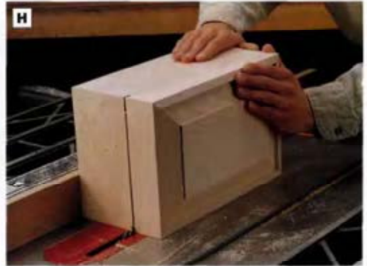
PHOTO H: Rip the box and lid into two pieces on the table saw, with the box bottom against the saw fence. Raise the blade to \frac{5}{8} in. and cut one end, then cut adjacent sides, working your way around the box.
