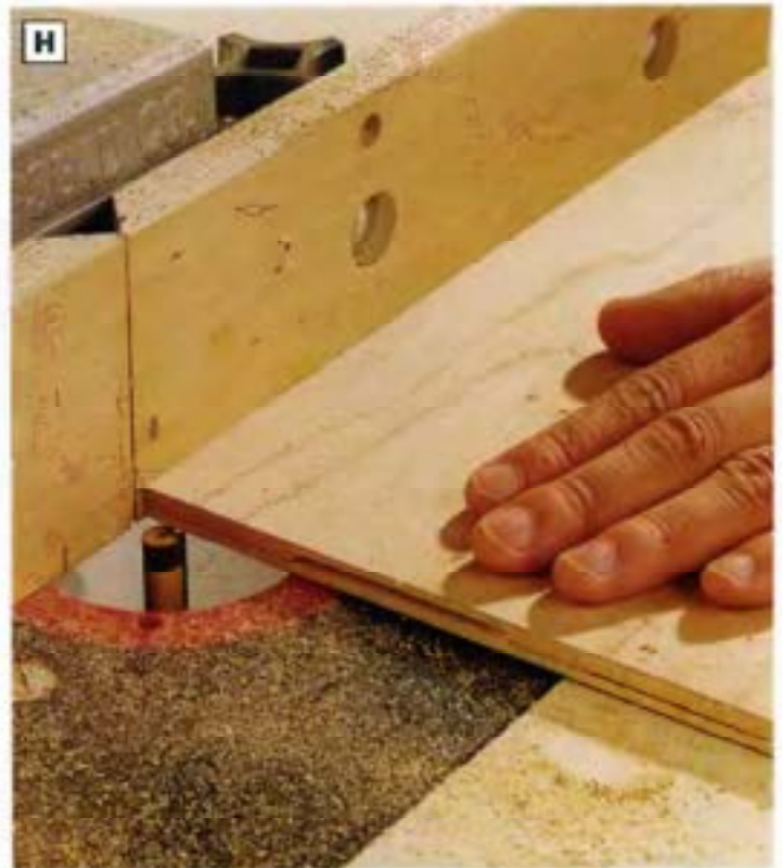
PHOTO H: Rout a shallow rabbet around the top face of the bottom panel for the veneer inlay strips. Install a \frac{1}{2} -in. straight bit in your router table to cut this \frac{1}{2} -in.-deep rabbet. Practice on scraps first and test the fit of the strips in the rabbet.
