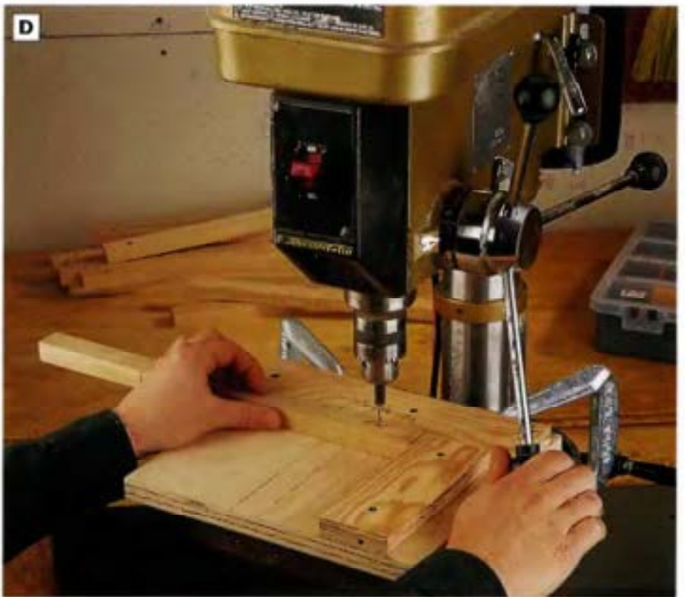
PHOTO D: Build a right-angle jig from scrap to help index placement of the counterbored holes in the ends of the slats. Clamp the jig to the drill press table so each slat is exactly aligned for drilling when you lay it in the jig. This way, there's no need to measure and mark each slat hole.
