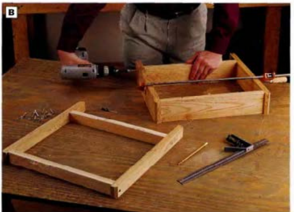
PHOTO B: Build an upper and lower frame for each chair. Note that the end pieces of each frame are inset \frac{3}{8} in. and 3\frac{1}{8} in. from the ends of the side pieces. Clamp the frame parts together, and drive 2-in. galvanized deck screws through the sides and into the ends to make the frames.
