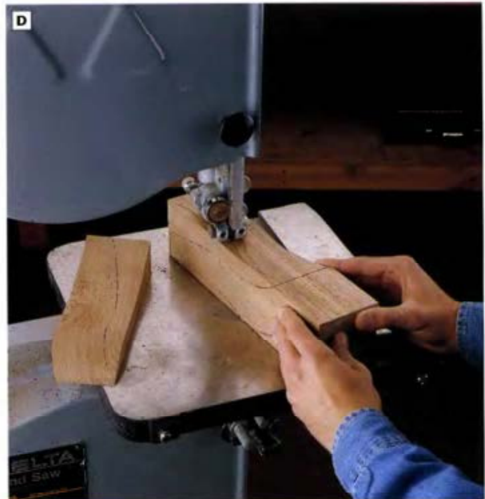
PHOTO D: Cut the profile on the adjacent side of each blank just as you did with the first side. The reattached waste pieces lend you flat surfaces for easier, accurate cuts.
