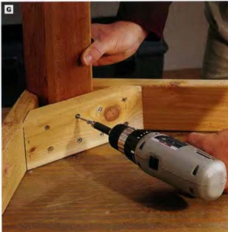
PHOTO G: Assemble the table legs, aprons and corner braces. Attach the parts by driving 2\frac{1}{2} -in. galvanized deck screws through countersunk pilot holes in the leg braces. Fasten the brace to each apron with a pair of screws driven in at an angle into the aprons, and use four screws for securing the leg. Be sure the legs are tight against the aprons and braces as you drive the screws.
