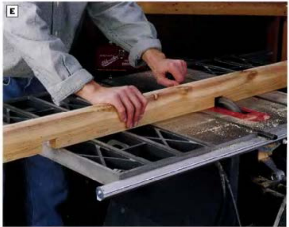
PHOTO E: Cut 1½-in.-wide notches on the top edge of the cross support. The notches fit together with the notches cut into the bottoms of the seat supports.
