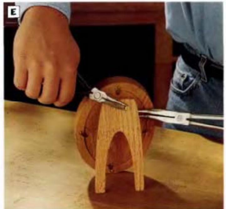
PHOTO E: After locating the hinge position, mount the hinge to the frame back with #4 x 1/4-in. brass flathead wood screws. Fasten the hinge to the stand with bolts and nuts. Arrange the bolts so you can thread the nuts on from the back of the stand. Tighten the nuts and bolts with a pair of needle-nose pliers.
