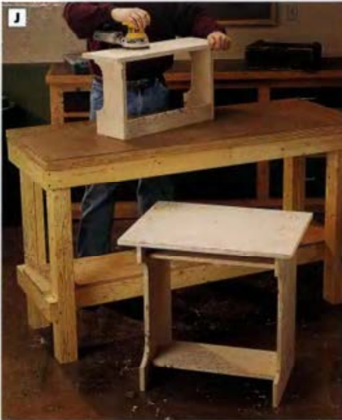
PHOTO J: Once you've filled all the screwholes and any voids in the plywood, sand the bench and desk before you prime and paint. A random-orbit sander and 150-grit sandpaper will make this a quick task.
