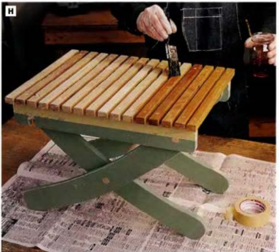
PHOTO H: Coat all raw wood, including the dowels, with Danish oil or another clear exterior wood finish to protect the wood from UV rays and moisture exposure. Use masking tape to keep painted surfaces clean when you brush the slats and dowels with wood finish.
