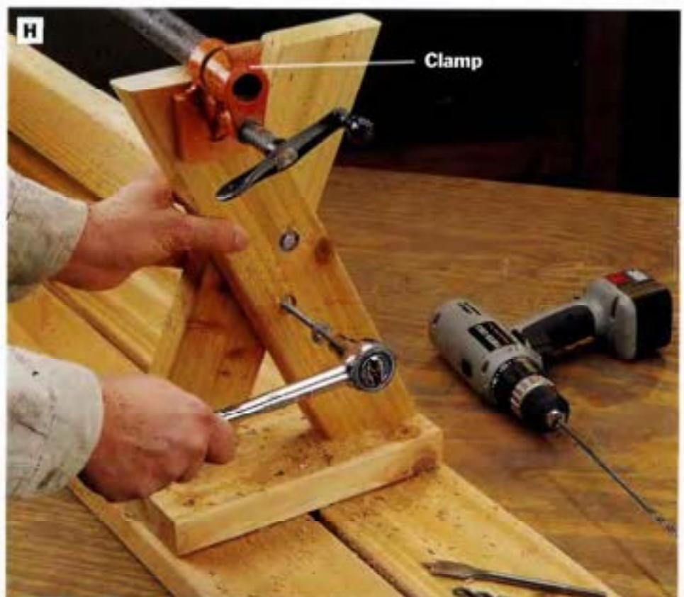
PHOTO H: Cut the bench braces to length and clamp them in position 5\frac{1}{2} in. from the bottoms of the legs on each bench. Drill \frac{3}{4} -in.-dia. counterbores in the outermost legs to recess two lag bolt heads, then drill pilot holes through the counterbored holes to install the lag bolts. Slip a washer onto each lag bolt before you screw it through the legs and into the bench braces.
