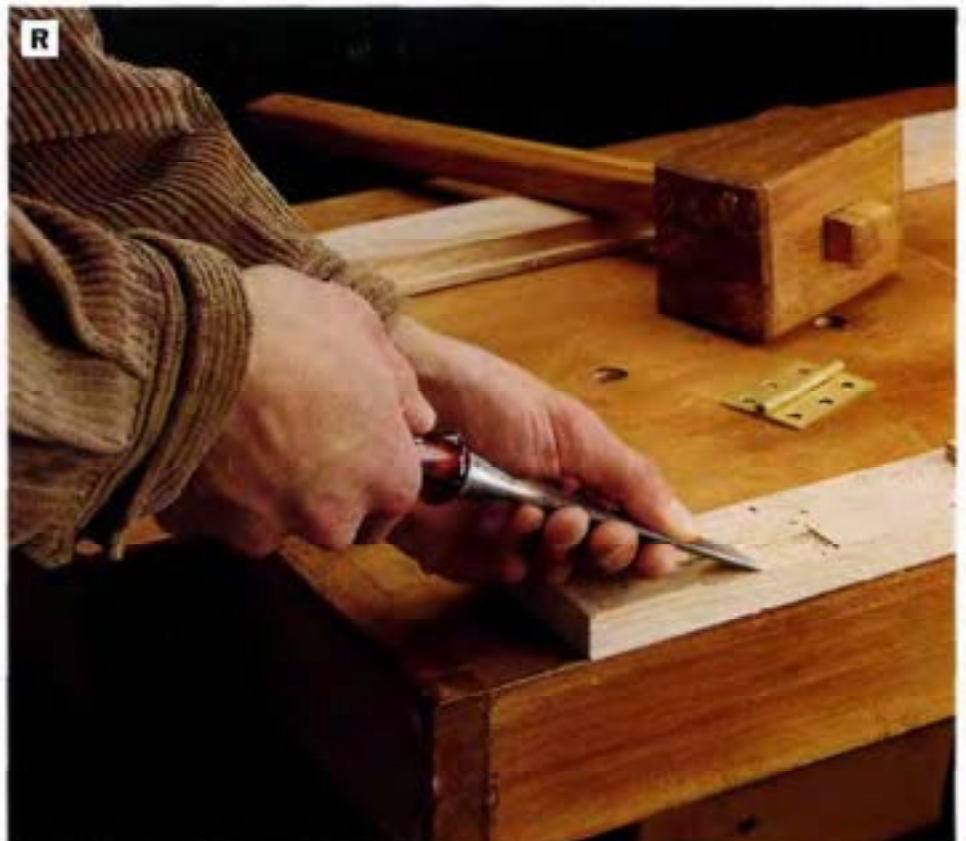
PHOTO R: Chisel mortises for the hinges into the inside faces of the outer door stiles and into the front edges of the cabinet sides. Use one of the leaves from the 2½-in. butt hinges as a template for tracing the cutting lines for the mortises.
