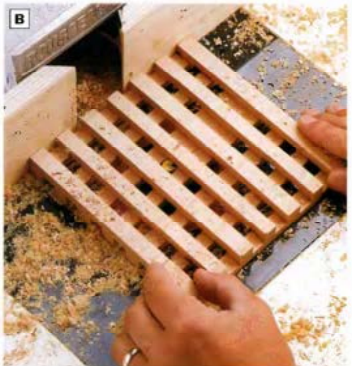
PHOTO B: Reposition the fence at 1\frac{1}{2} in. and 2\frac{1}{2} in. from the bit for the second and third rounds of cuts. Continue milling the grooves in three passes, raising the bit after each, until the trivet is completed.
