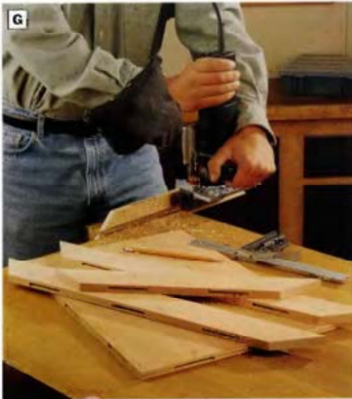
PHOTO G: Lay out and cut #20 biscuit slots to join the frame side and end pieces to the bottom panel. Clamp the parts in a bench vise to hold them securely when you cut the slots.
