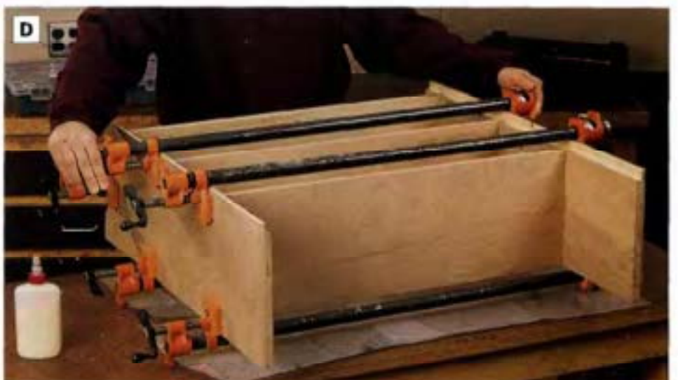
PHOTO D: Glue and clamp the shelves into their dados in the bookcase sides. Keep the shelves flush with the front edges of the sides so they don't obstruct the back rabbets.
