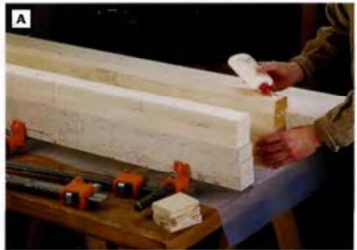
PHOTO A: Face-glue the benchtop in sections of four or five boards, then face-glue the sections together.
