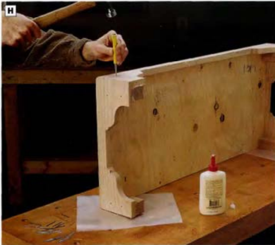
PHOTO H: The trim pieces wrap around the base structure, adding decoration and “feet” to the cabinets. Use 4d finish nails and glue to attach the mitered trim pieces. Drill pilot holes for the nails (you can remove the head from a finish nail and chuck it into your drill if you don’t have a drill bit small enough for the job). Set nails with a nailset.
