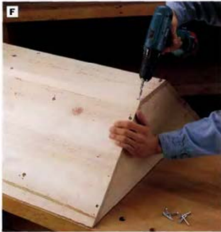
PHOTO F: Assemble the carcass parts using 1½-in. flathead wood screws to reinforce the joints. Attach the cupboard back by driving the screws at an angle through the back and into the sides.
