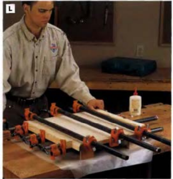
PHOTO L: Glue and clamp the edging to the tabletop, using #20 biscuits to keep the parts aligned. Match up the miters. NOTE: The long miters on the wider front edging will protrude past the sides.
