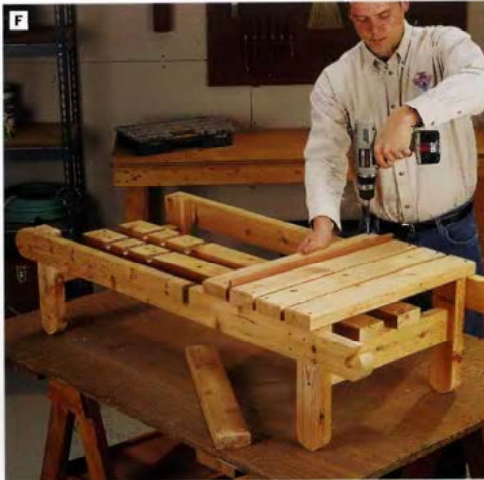
PHOTO F: Screw the five seat slats to the seat rails. Determine and mark the positions of the end slats first, then space the remaining three slats evenly between the end slats. If the slat space is consistent on your chair, use a scrap spacer to make spacing easy when fastening the parts.
