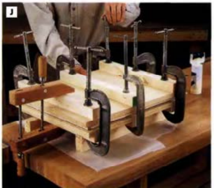
PHOTO J: Clamp the veneer to the glued-up panel in a homemade caul-and-particleboard plate veneer press. Allow a few minutes for the glue to squeeze out, then check to see if the clamps need tightening again. Let the glue dry for at least four hours before you remove the veneered panel from the press.
