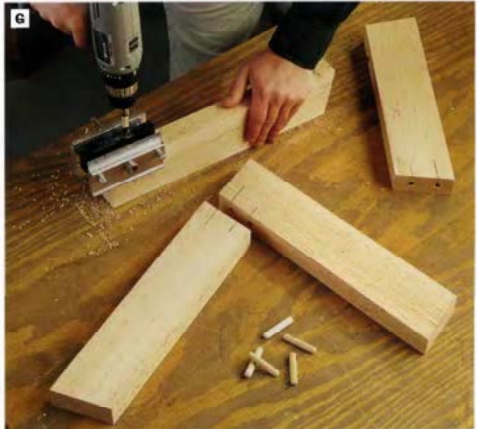
PHOTO G: Join the bench legs to the arm supports with pairs of 2-in. fluted dowels. Use a doweling jig when you drill the holes to be sure that the dowel holes are drilled straight across the joints. Wrap a piece of tape around the drill bit to serve as a temporary depth stop.
